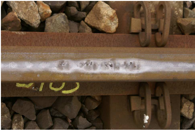
Fig 1: Example of severe squats on a rail
