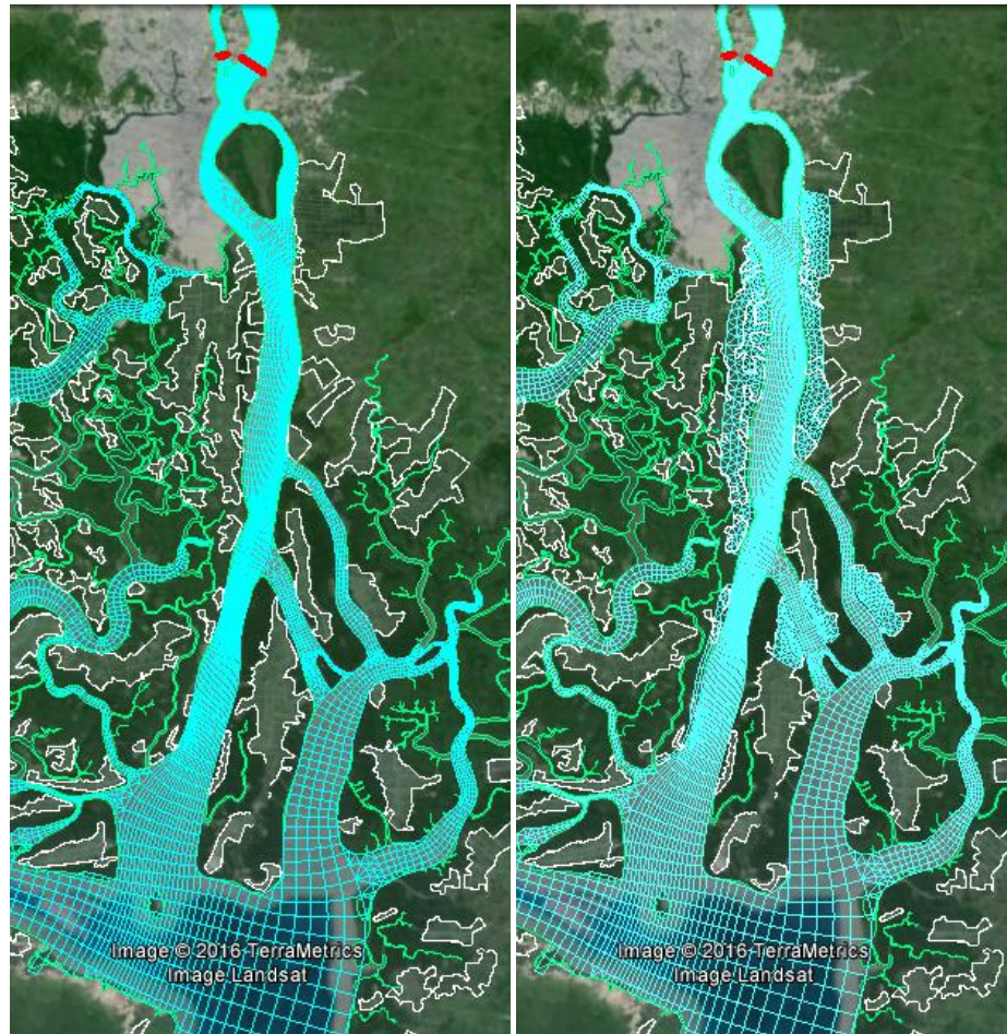
Figure 6.1: Reference (left) domain and modified (right) model domain (light blue) that includes the intertidal and mangrove forest areas currently occupied by shrimp farms (white). 'Puente de la Unidad Nacional' bridge (red)
