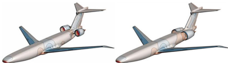
Fig. 1 NOVA aircraft configurations: conventional w.rear fuselage engines and BLI configuration
