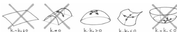
Figure 1: Design guidelines for irregular double curved shell [8]
