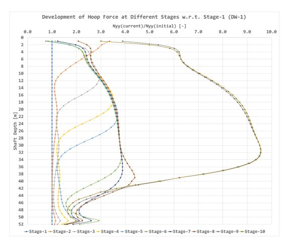
Figure 5-7: Comparison of current:initial hoop force at different stages (3D, DW-1)
