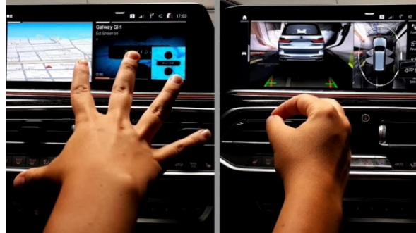
Figure 9 – Use of hand gestures for interaction with HMI, BMW X7 (Cardesign use, 2019)
