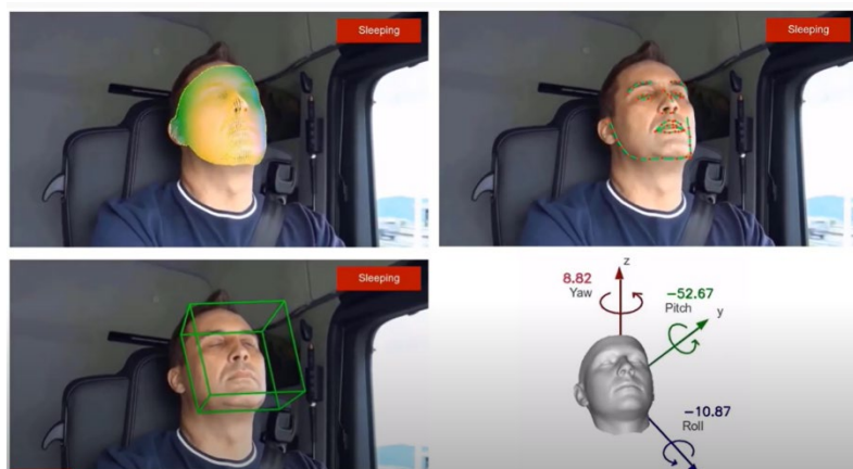
Figure 15 - An example view of cameras used for Driver Monitoring, developed at the University of Leeds (Rezaei, 2021).
