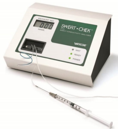
Figure 3.2: Sweat-Chek™ Analyzer using ion conductivity technique [66]
