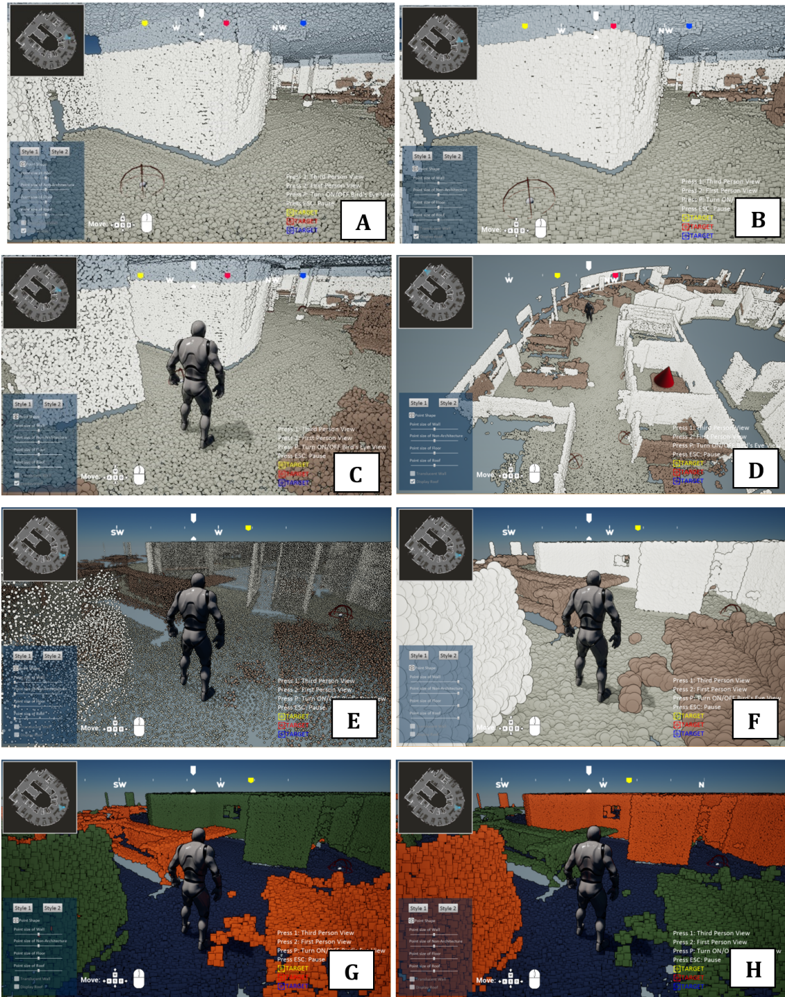
Figure 28: Some visualisation results: (A) View the point cloud data in first-person perspective, and the shape of the points is set as circles. (B) View the point cloud data in first-person perspective, and the shape of the points is set as squares. (C) View the point cloud in third-person perspective. (D) View the point cloud data in bird's eye view, the positions of the avatar and the red target can be identified. (E) Set the point size as the smallest size. (F) Set the point size as the biggest size. (G) View the point cloud in style 1. (H) View the point cloud in style 2.
