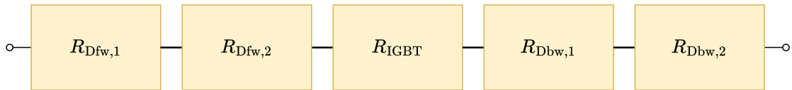
Figure 4.10: Reliability block diagram of the SSCB describing a series reliability network.
