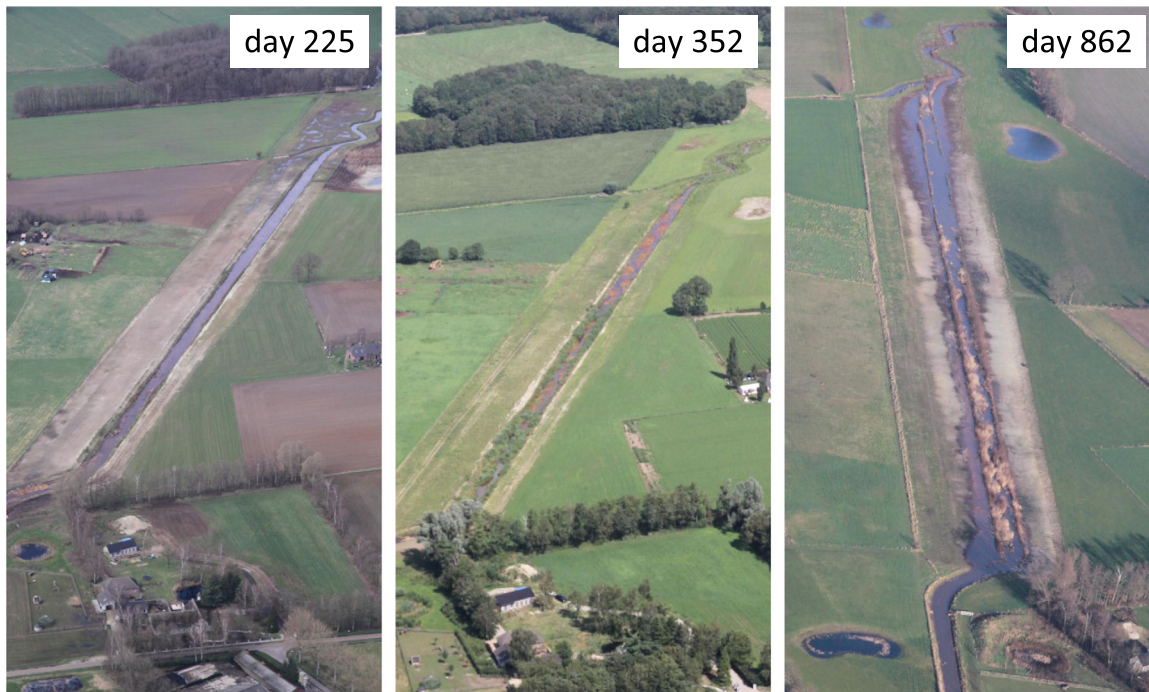
Figure 3. Aerial photos of the experimental reach, taken at 225, 352, and 862 days after the start of the experiment. Water is flowing from the bottom to the top. The middle photo shows a clear difference between the vegetated area (upstream) and the regular pattern of alternate bars (downstream).
