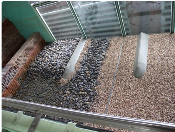
Figure 6.2: Upstream inflow boundary with increased roughness to distribute the discharge between the main channel and groyne field.
