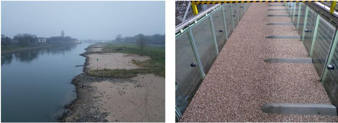
Figure 6.1: The River IJssel (left) during extremely low discharge in November 2018 and the BAW flume (right). The difference in bed level of the groyne field can clearly be seen. Also the difference in bed roughness between the groyne and groyne field can be seen.
