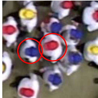
Figure 6.4: Two pedestrians walking close but not colliding in the evacuation experiment. The circular body formulation in Nomad predicts a collision.
