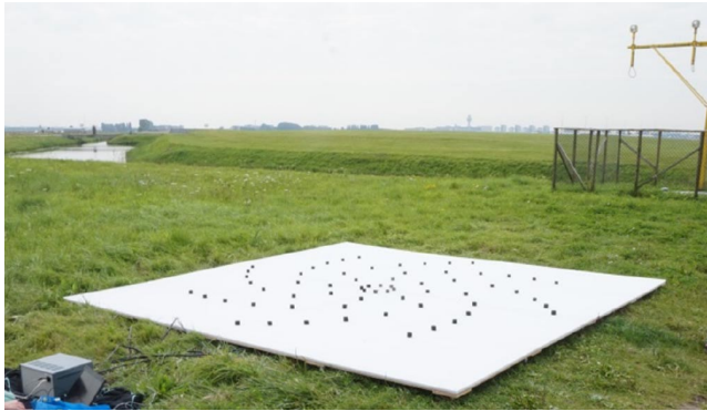
Fig. 2 Acoustic camera used to record the flyovers at Amsterdam Airport Schiphol.
