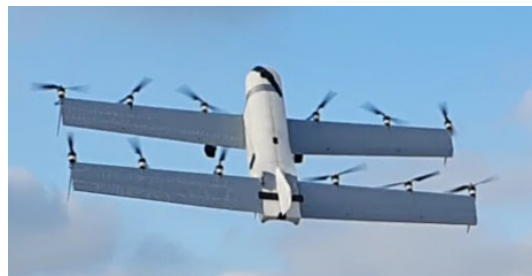
Figure 1: The Nederdrone, capable of performing VTOL. The tailsitter has 20 actuators (12 motors and 8 elevons) and the energy is stored in a hydrogen tank.
