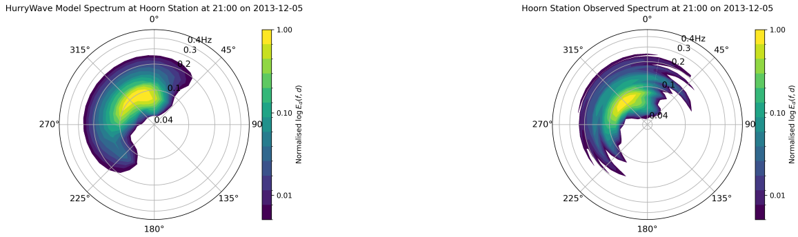
Figure 4.38: Comparison of directional-frequency wave spectra from HurryWave (left) and spectral buoy data (right) at Hoorn Q1-A on 5 December 2013 at 21:00. Both plots represent the late stages of the Sinterklaas storm's directional transition from North West to north. The model's slower response to changing wave direction suggests limited coupling between evolving wind conditions and wave propagation.
