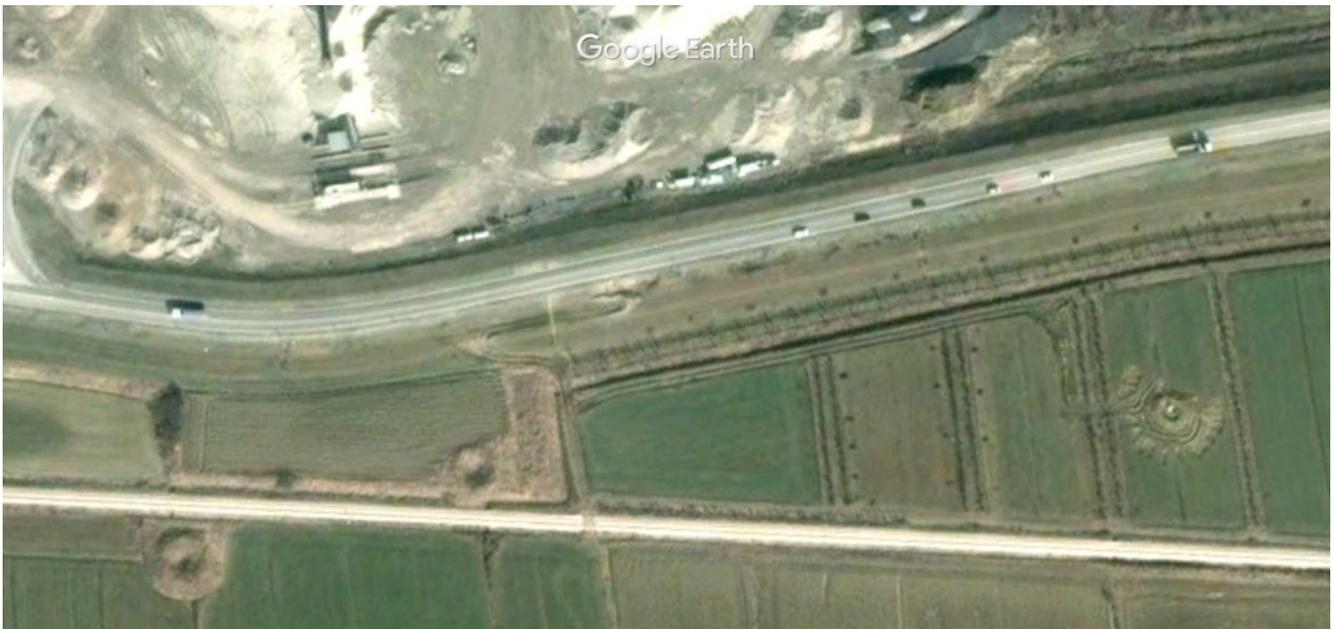
Figure 7. Sand Boils near the river Po, Boretto, Italy, 2003. (Picture Google Earth, 2003)
