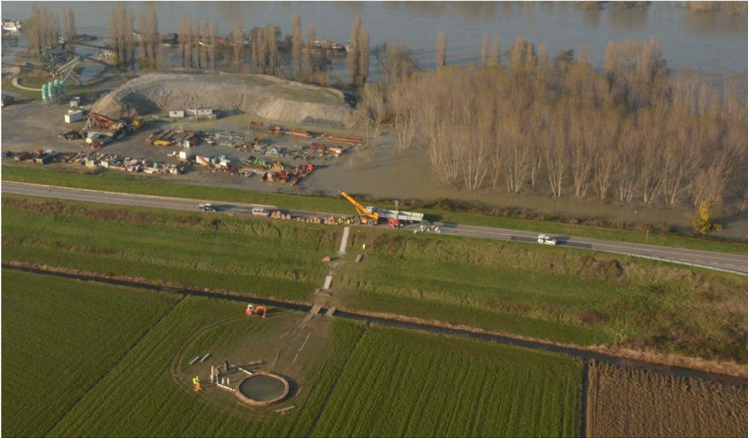
Figure 3. Ringed sand volcano near Boretto (Courtesy of AiPo).
