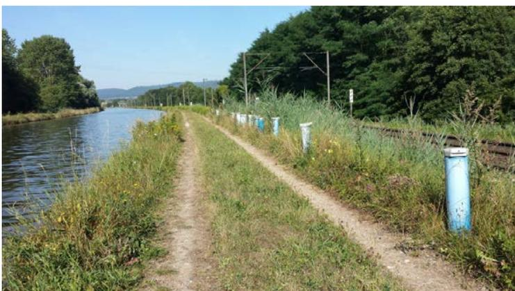
Figure 2. Array of temperature probes along the downstream side of the dam's crest, equipped with protecting devices containing dataloggers sending the monitored data to the office via remote transmission.
