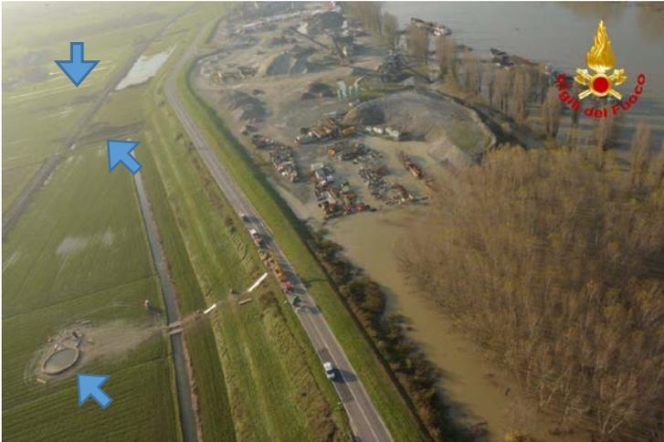
Figure 1. Piping along the Po river. Apart from the 'fresh' sand boil on the left part of the picture two older sand boils can be seen (sand boils indicated with arrows).
