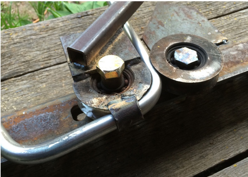
Figure 77. Bending a metal pipe
