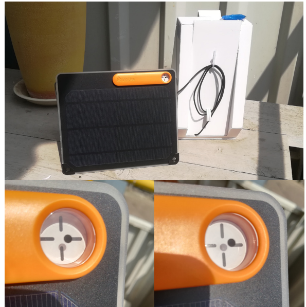
Figure 83. BioLite solar panel, including sundial On the Left: Wrong position; On the right: Correct position
