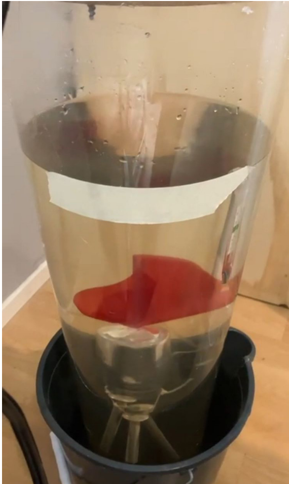
Figure 23: A pressure chamber was constructed to do more controlled tests
