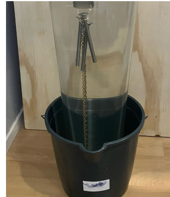
Figure 48: A chain helps compensate forces for higher pressure at depth
