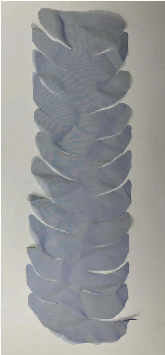
Figure 50: Cutting pattern for the flaps in the fabric
