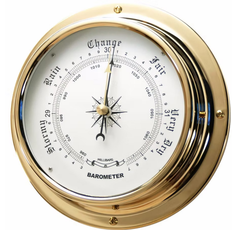
Figure 4: A classic aneroid barometer (Olorvida, 2021)
