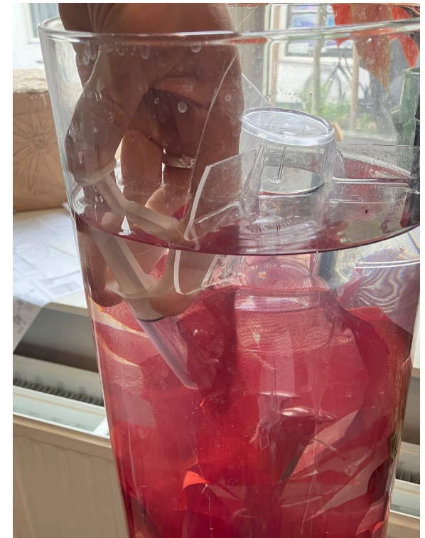
Figure 44: Filling the diver with air to make it just float
