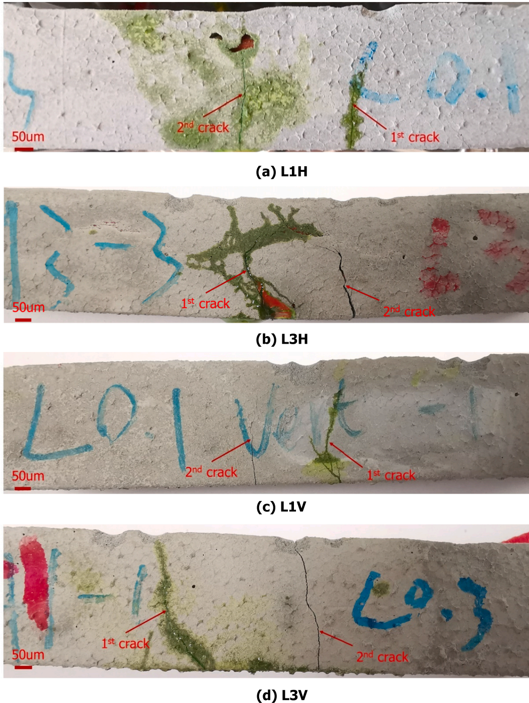
Fig. 17. Crack morphology after the second 4-point bending test (a) L1H; (b) L3H; (c) L1V; (d) L3V.
