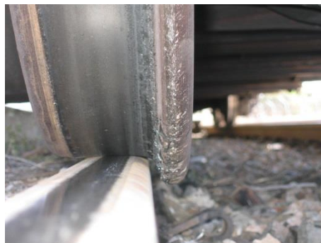
Figure 3.5 Interaction between rail and wheel that provides guidance
