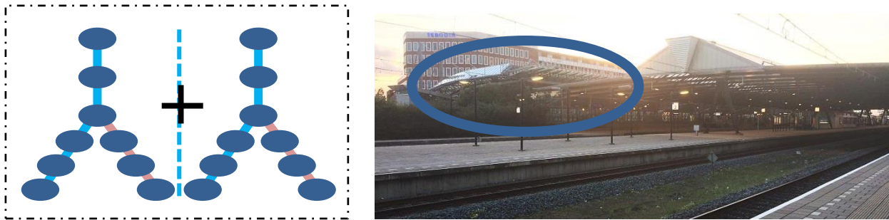
Figure 4.9 Level 4 untangling: two systems function completely independently. Example Rotterdam metro and national rail systems meet in Schiedam Centrum station
