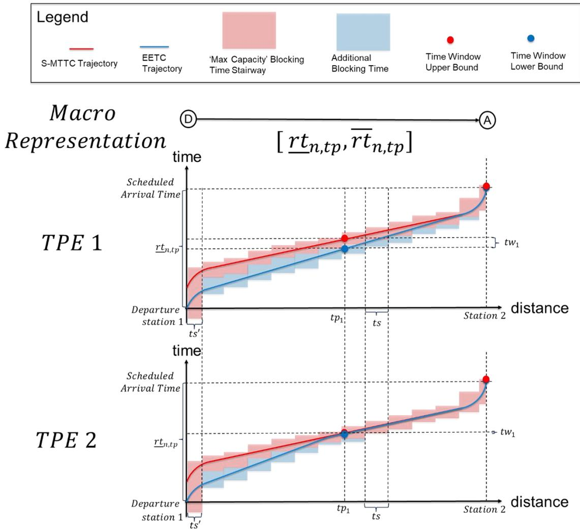
Figure 7: Blocking time diagrams train path envelopes showing the blocking time stairway that maximizes theoretical capacity (red) and additional blocking time (blue) for energy-efficient train control
