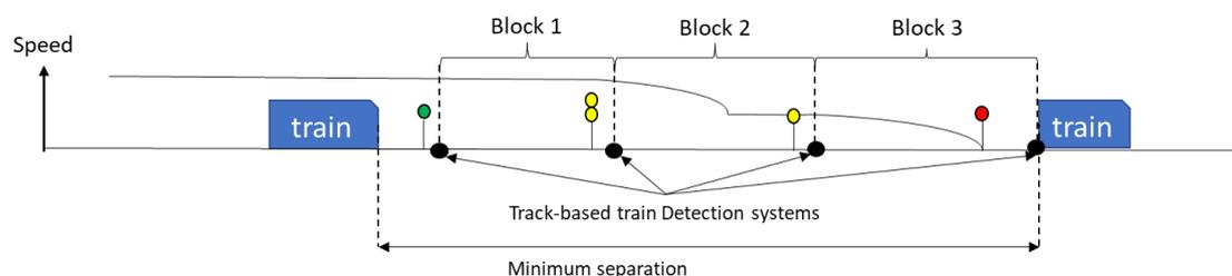
Figure 2: Minimum following distance for standard sequence UK four-aspect signalling (adapted from Busuttil, 2023)
