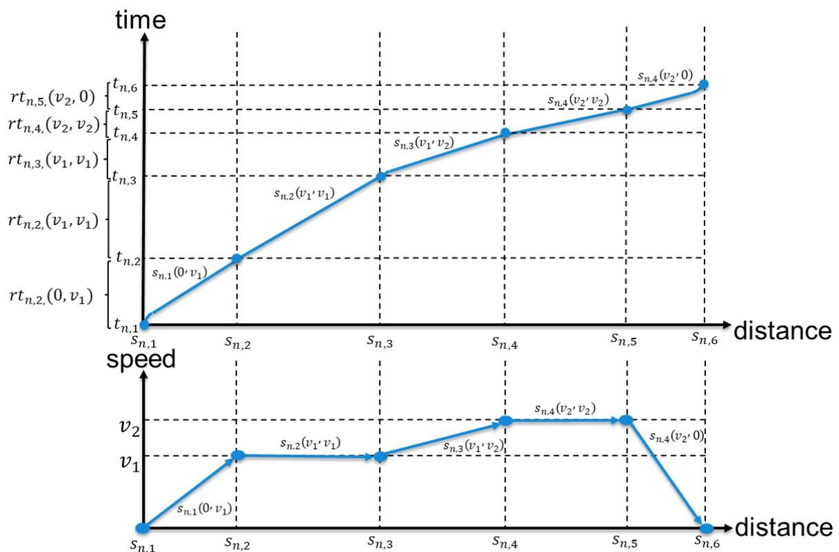
Figure 8: The relationship between speed-distance arc selection and the time-distance trajectory
