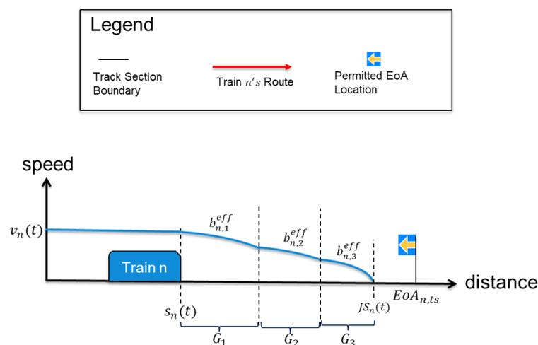
Figure 12: The impact of changes in track grade on the effective braking rate and the job-start frontier location
