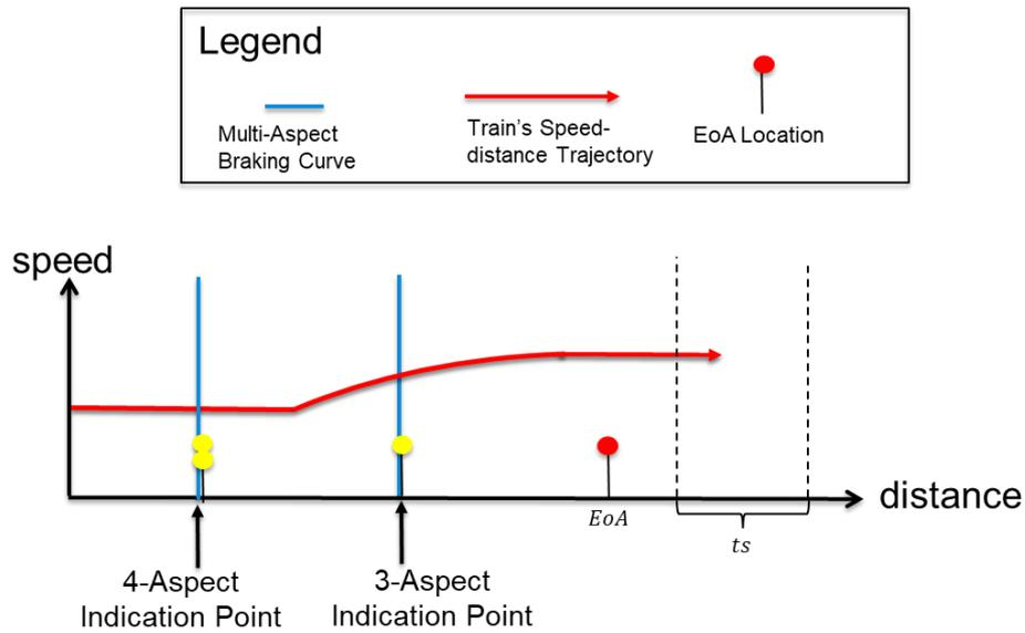
Figure 14: Derivation of three- and four-aspect indication points for a track segment for a fixed trajectory.
