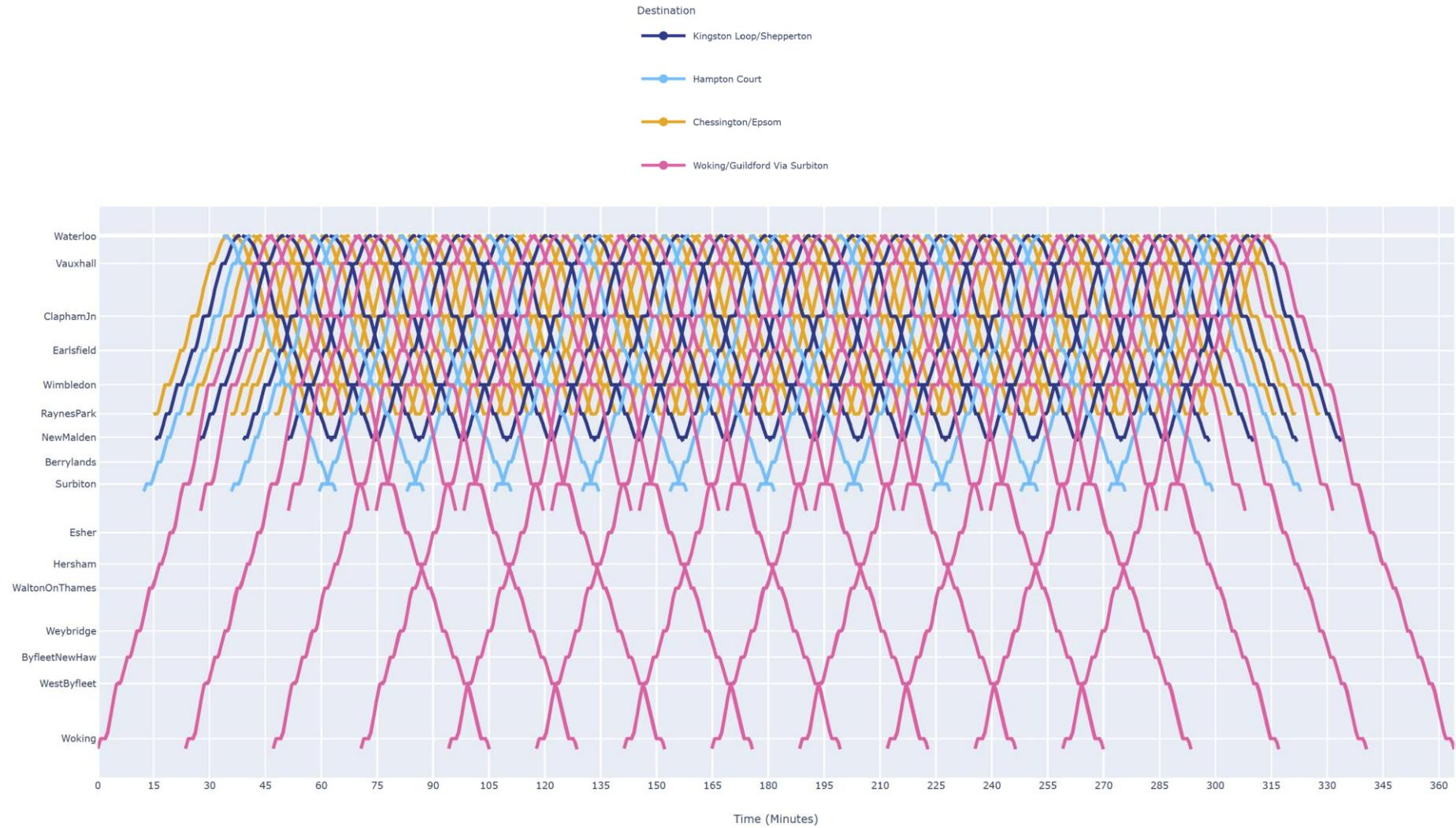
A.2 Results for Main Slow Line with three-aspect Signalling (6 Cycles Shown)
