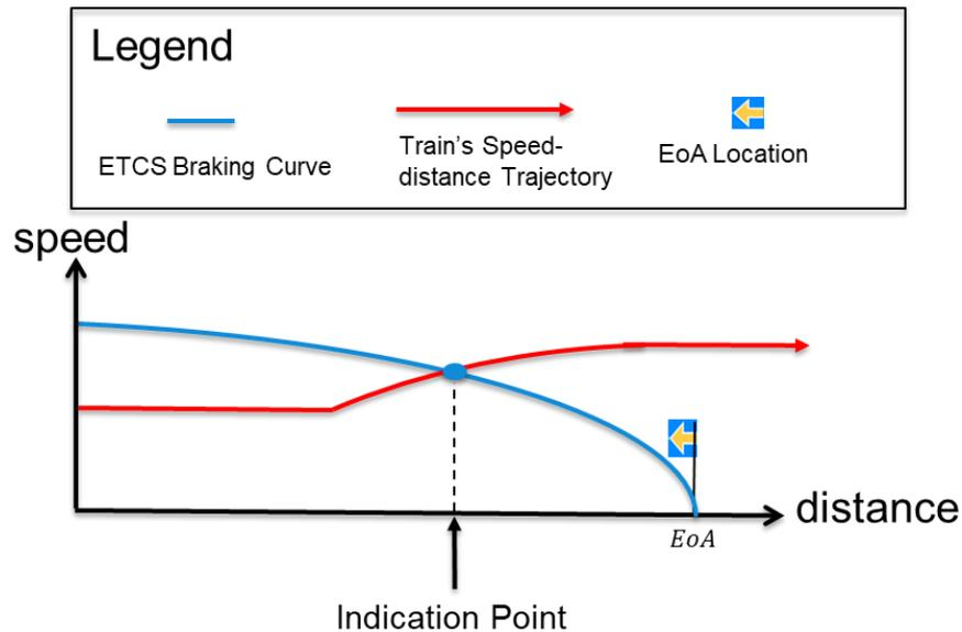
Figure 13: Derivation of ETCS full supervision indication point for a track segment for a fixed trajectory.
