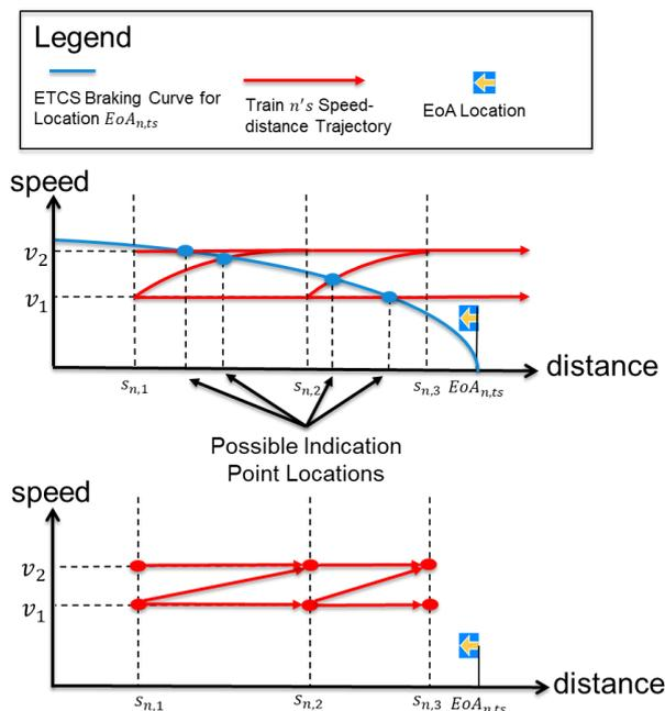
Figure 15: Impact of Speed-distance arc chosen on the interval the indication point occurs in.
