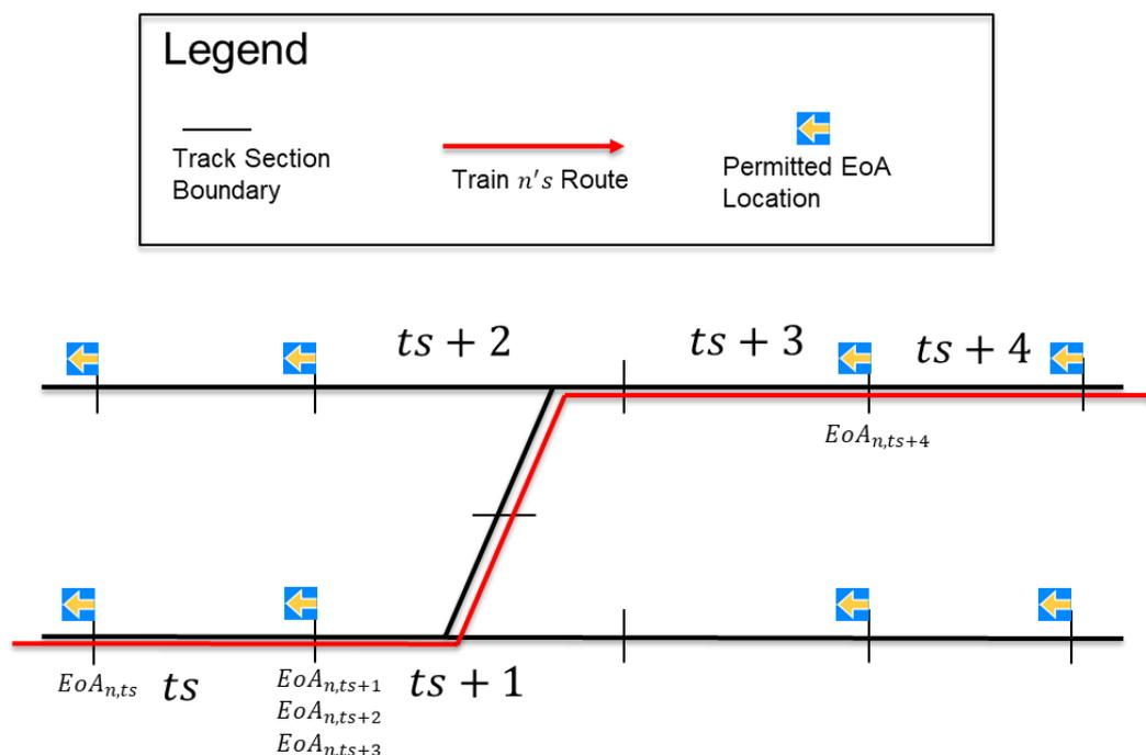
Figure 10: Placement of reservation start locations in Interlockings with Sectional Route Release
