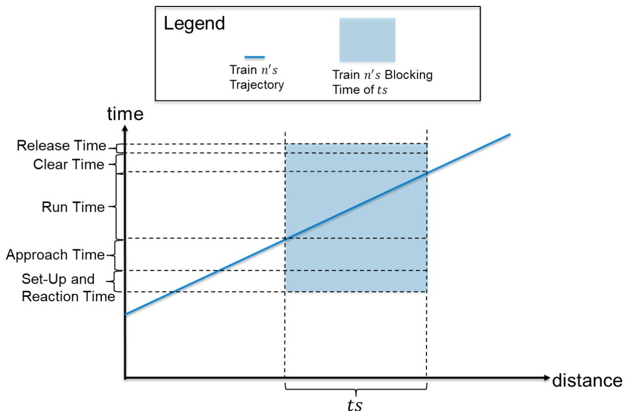
Figure 5: Components of Blocking Time Calculations
