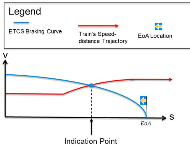
Figure 3: Calculation and Supervision of the braking curve in ETCS
