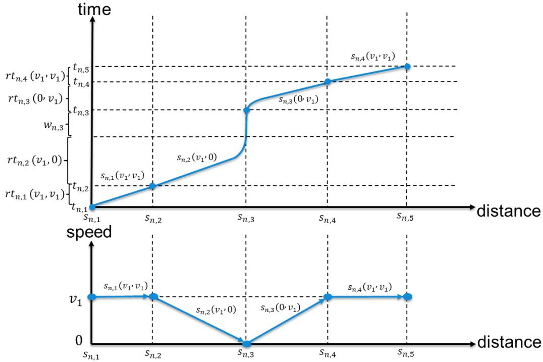
Figure 9: The relationship between speed-distance arc selection and the time-distance trajectory when a train stops and waits at timepoint 3
