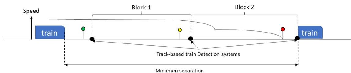
Figure 1: Minimum following distance for three-aspect Signalling (adapted from Busuttill, 2023)
