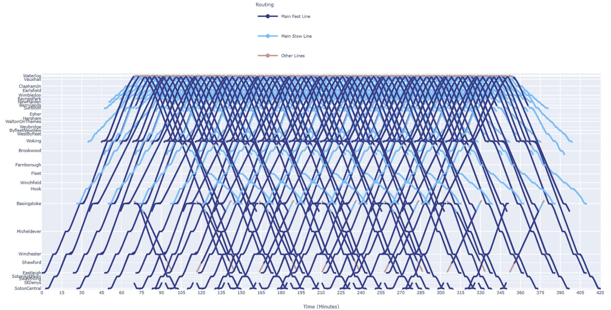
A.4 Results for Whole South West Main Line with Mixed signalling (6 cycles shown)
