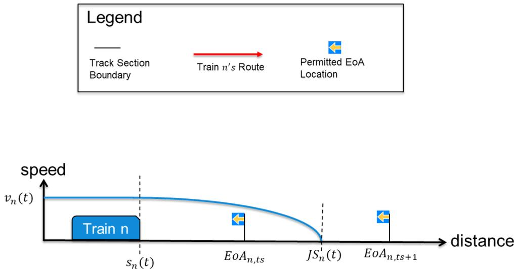
Figure 11: Visualization of the Job-start frontier of train  $n$  at time  $t$  in relation to the position of its head
