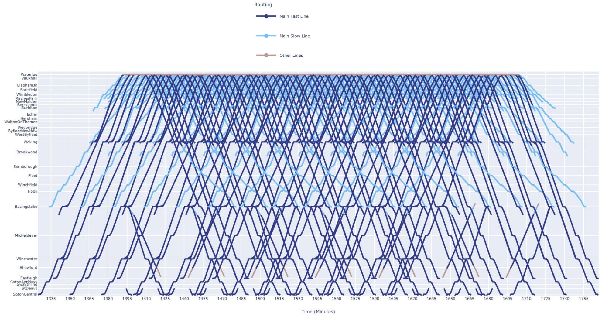
A.3.4 Minimized Cycle Time with No Turnaround Constraints
