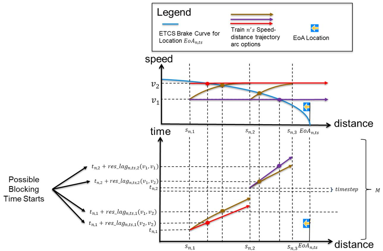
Figure 16 : Relationship between speed-distance trajectory selection and exact reservation start times, with  $M$  and timestep shown for scale. Only arcs with a reservation lag other than  $M$  or  $-timestep$  are shown in the time-distance diagram.
