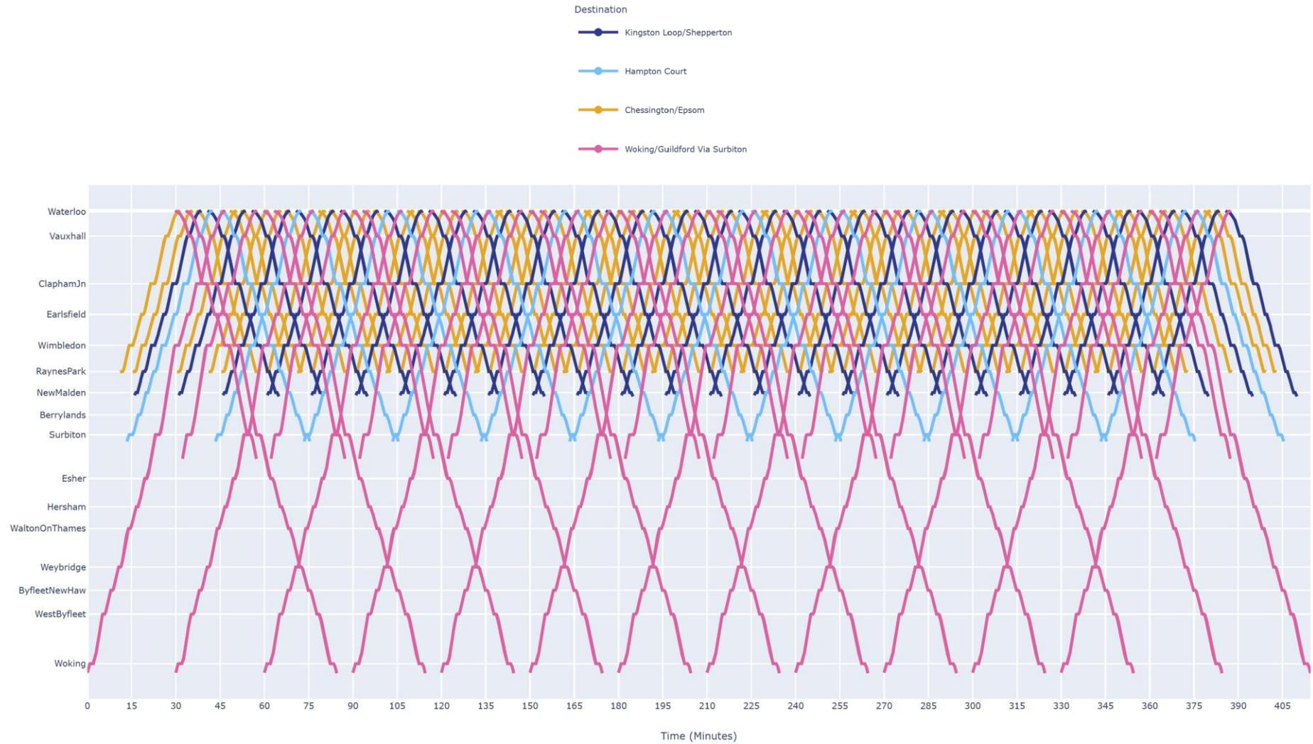
A.3 Results for Whole South West Main Line with ETCS Level 2 signalling (6 cycles shown)
