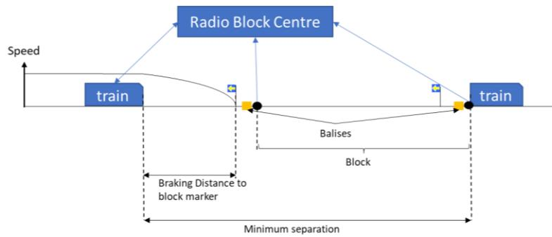
Figure 4: Architecture of ETCS Level 2 Signalling (adapted from Busuttill, 2023)
