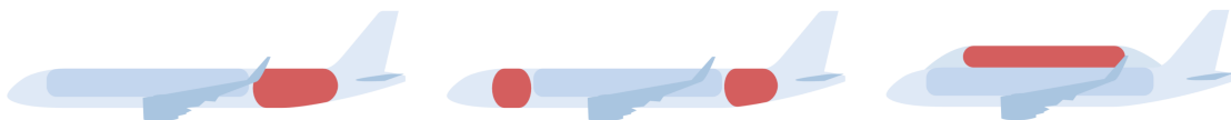
Figure 2.3: Possible hydrogen tank configurations for tube+wing aircraft, where the darker shade of blue represents the passenger cabin. Image obtained from Adler and Martins [8].
