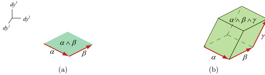
Figure 2.12: 2.12(a) The exterior product of two 1-forms \alpha and \beta yields the 2-form \alpha \wedge \beta . 2.12(b) Multiplying by yet another 1-form \gamma give the 3-form \alpha \wedge \beta \wedge \gamma
