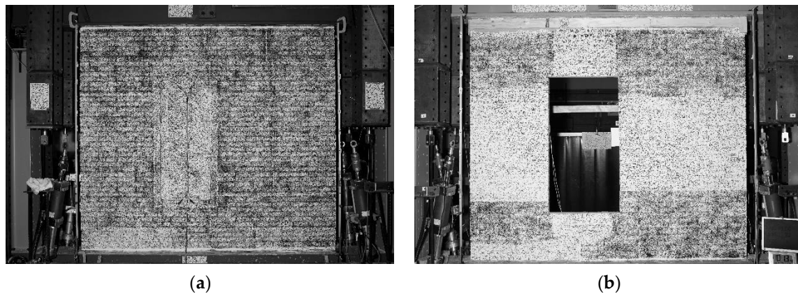
Figure 4. Front view of the in-plane walls with the DIC black-and-white pattern applied: (a) strengthened (TUD-COMP56) and (b) unstrengthened (TUD-COMP41) specimen where the glass and timber frame are also painted.
