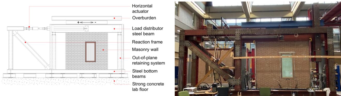
Figure 6. In-plane test set-up looking at the back of the wall (without DIC pattern).
