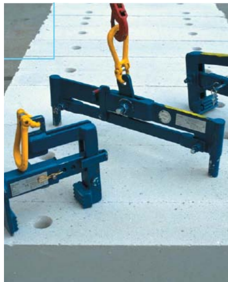
Fig 97: mechanical lifting and placing of a panel 24
