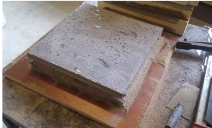
Fig 169: First panel deshuttered
