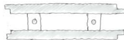
Fig 135: Sketch of plan of the panel incorporating the sleeve for the bolt in the shear connector
