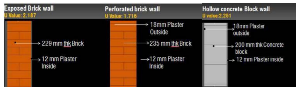
Fig 141, 142: U values of typical conventional walling systems
