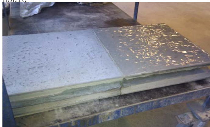
Fig 171: trial of horizontal assembly of 2 panels
