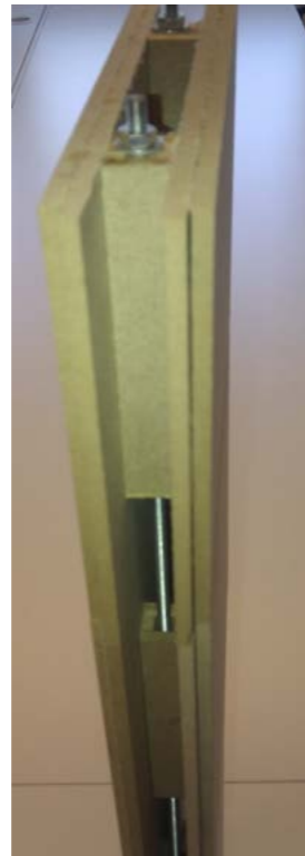
Fig 133: section and elevation illustrating the prestressing of panels with bolts as an idea
