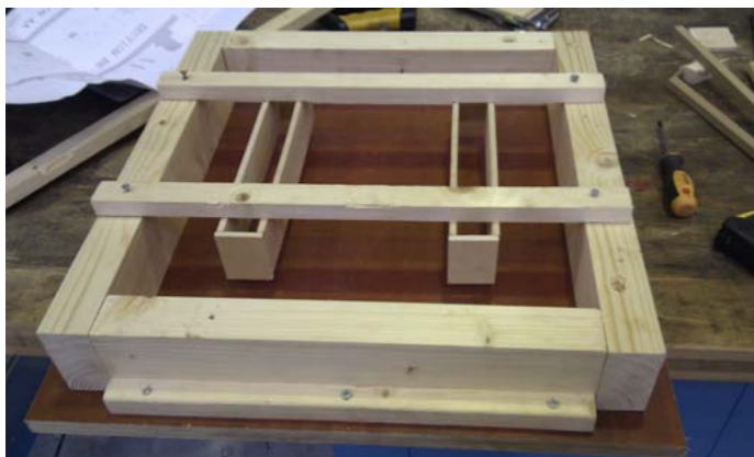
Fig 162,163: Views of completed mould
