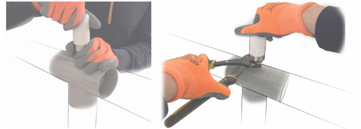
Figure 40: Edge Dynamics pressure sensor mounted, unscrewing by hand (left), unscrewing using tool right)
