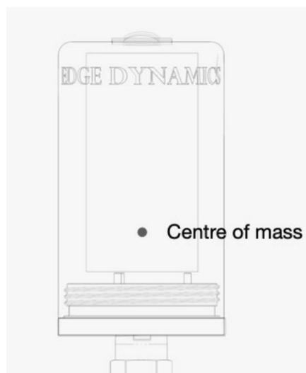
Figure 5: Centre of mass of current sensor node
