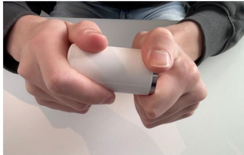
**Figure 36: The surface area of the base is small (steel part in hand on the right). Exerting the required force on the sharp edge of the base is uncomfortable.**
