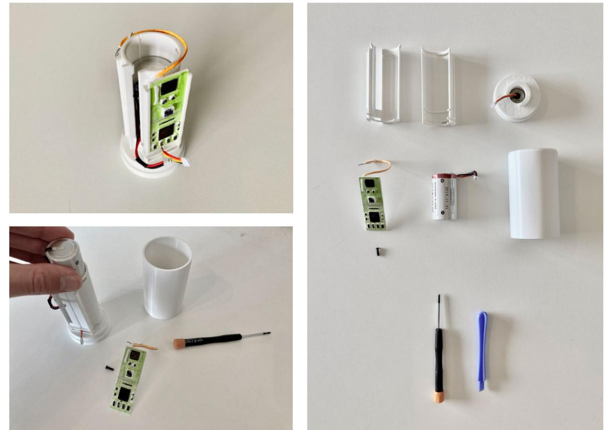
Figure 73: (Clockwise, starting top left) assembled prototype; disassembly of battery, full disassembly
