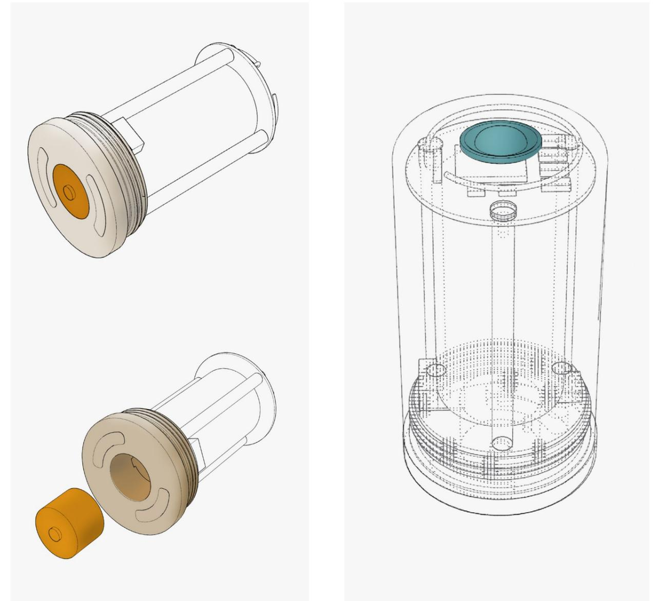
Figure 42: Left; Coupling between base and sensor insert, Right; coupling between button and casing
