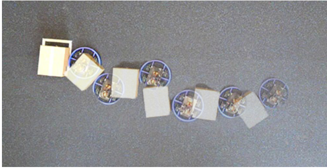
Figure 5.1: Manipulating object to the goal with a low-cost mobile robot: Mirte Master. The transparency of the robots and boxes indicates their movement.
