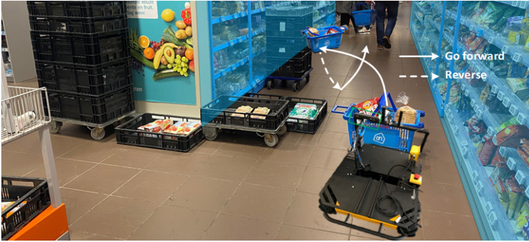
Figure 1.1: A Husky robot navigating a supermarket environment encounters baskets blocking its path. To clear the way, it attempts to push the baskets aside before reversing to realign with its predefined path.
