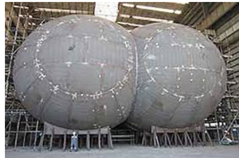
(b) Bilobe tanks (largest tanks in 2013) built at Chinas Sinopacific yard [2]
