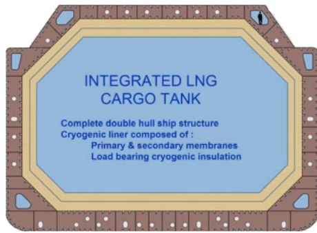
(a) Architecture of the membrane tanks [17]
