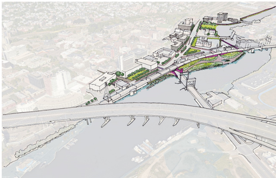
Fig. 6. Conceptual design with eco-engineering applications to produce a hybrid design to enhance resilience in an urban center (Bridgeport, Connecticut, USA) and ultimately protect critical infrastructure, public amenities, and utilize natural systems to both accommodate flooding and reduce risk in response to flooding from sea level rise and Category-3 hurricane (i.e. “resilient triple bottom line”). Design integrates typologies from Figs. 1 and 2 including flood water retention, bioswales, green streets, living shorelines, and obstacle removal. (Credit: The Nature Conservancy & Urban Ecology and Design Laboratory – Yale University; [100]).
