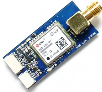
Figure 9: The chosen GPS model, NEO-7N GPS module.
