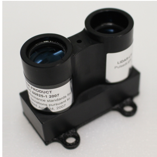
Figure 12: The LIDAR Lite Sensor
