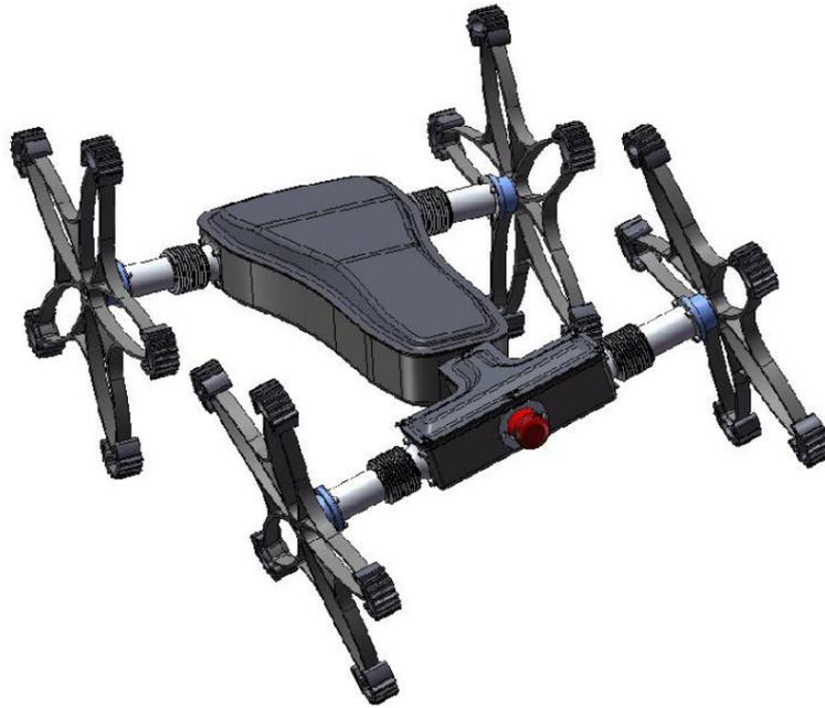
**Figure 1-3:** CAD model of the Asguard II robot from DFKI.
