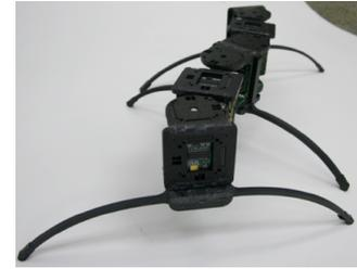
**Figure 1-6:** CKbot legged configuration.
