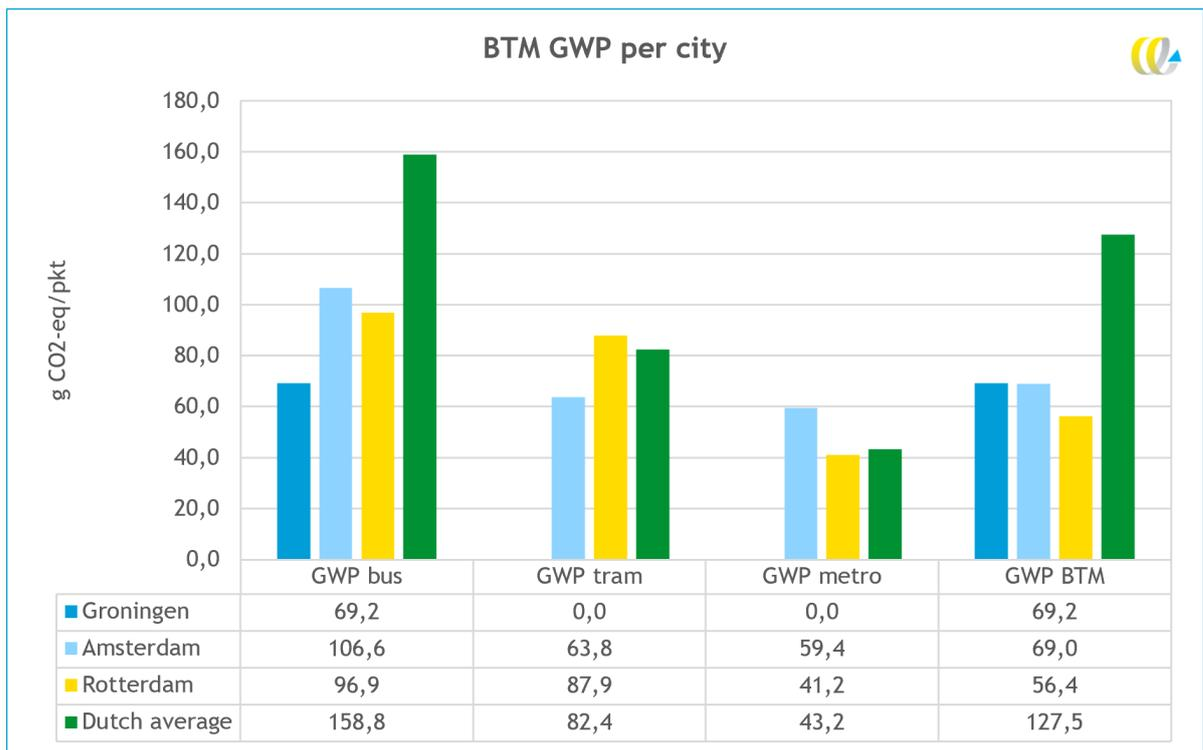
Figure 7.7: GWP of bus, tram and metro and BTM combined for the four case studies
