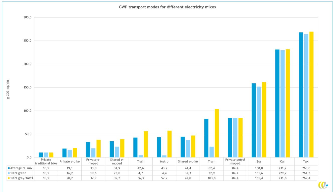
Figure 7.12: Sensitivity Analysis: Electricity mix
