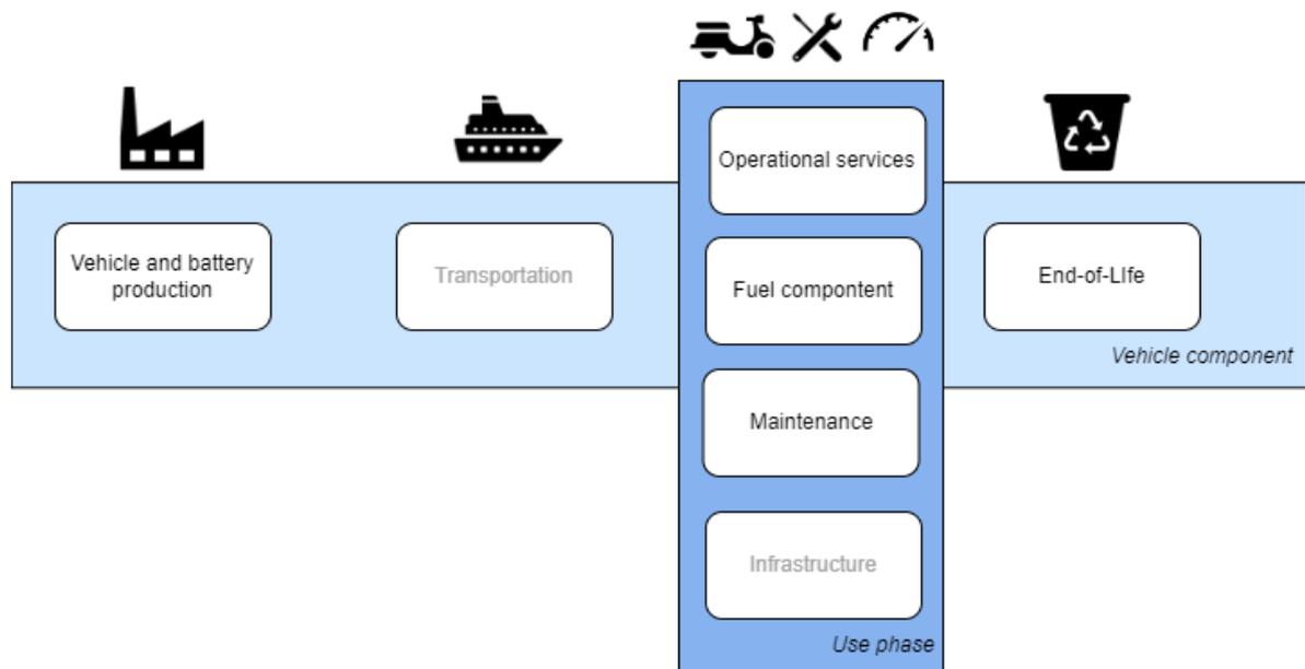
Figure 5.1: LCA components for shared e-mopeds. Light grey boxes - transportation and infrastructure - are neglected in this study. Own illustration based on all reviewed papers
