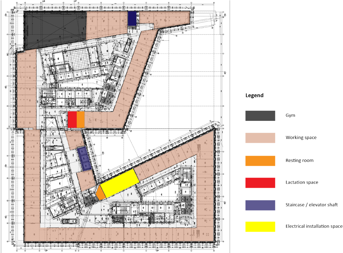
Fig. 13 Floorplan 6 th floor JuBi Towers and corresponding functions near the façade (BIM-model JuBi towers)
