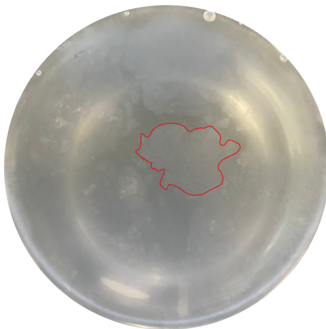
Figure 2.23: Alumina platelet with excessive platelet number. It is possible to see a heterogeneous film with darker portions that indicate multiple layers of platelets, like the one highlighted in red.
