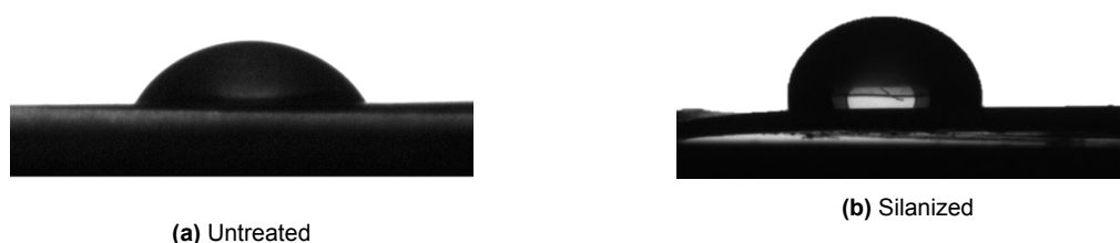
Figure 2.29: Water contact angle of coating with untreated and with silanized alumina platelets.
