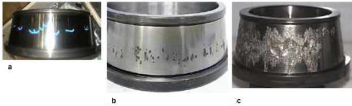
Figure 3.30: Failure appearance: a) straight cracks; b) straight cracks and small spalls; and c) spalls. [69]
