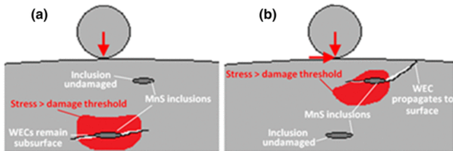
Figure 3.35: Importance of surface traction (not to scale): (a) pure rolling: critical stress threshold exceeded relatively deep—micro-cracking at inclusion may never reach surface and cause failure; (b) rolling and sliding: critical stress field shifted closer to surface—micro-cracking at inclusion propagates to surface, leading to failure [74]
