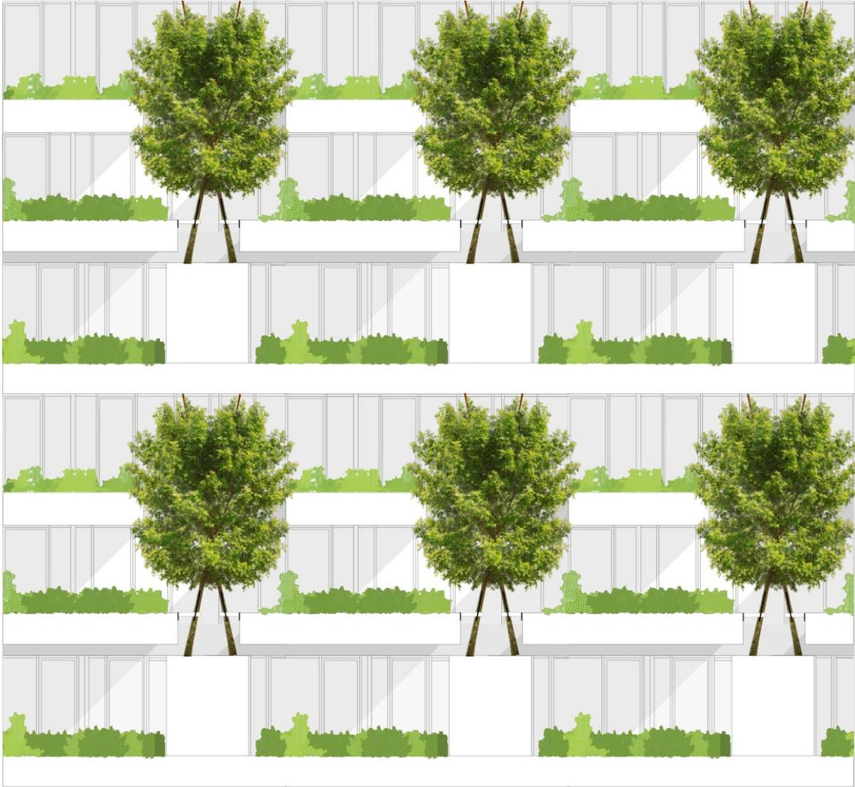
*Figure 8.7 Front view of Wonderwoods facade with plant containers connected to interconnected trees*
