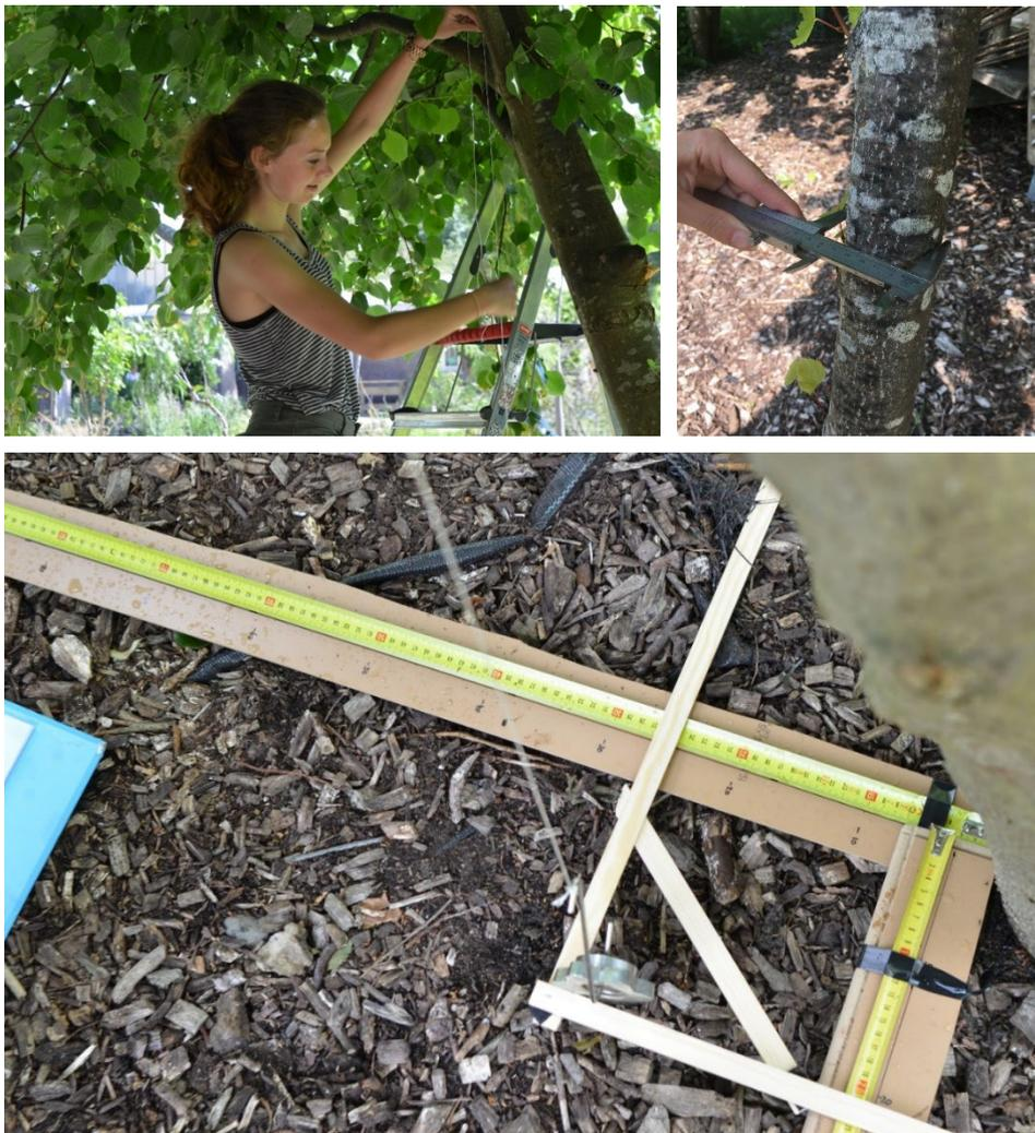
Figure 6.8 Geometry measurements. Top left: Measuring the height. Top right: Measuring the tangential width. Bottom: Measuring the radial and tangential coordinates.
