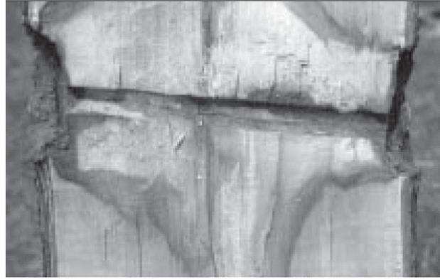
Figure 8.18 Left: Illustration of bolt going through the stem (Wahlländer, 2020). Right: Bolt created discolouration and white rot some years after installation (Stobbe, Dujesiefken, & Schröder, 2000)
