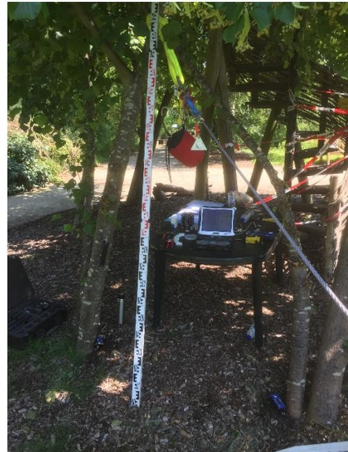
Figure B.12 Winching test set-up tree 9B-10A. Top left: Two measurement rounds and their elastometer locations. Top right: Top view with winching direction. Bottom left: Force is applied at the connection. Bottom right: Photo of set-up.
