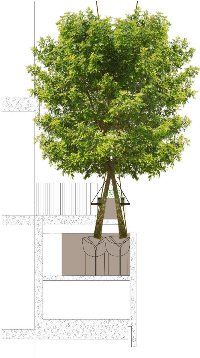
*Figure 8.8 Side view of interconnected trees in a tree container with root ball anchoring. The trees are connected to a plant container with brackets and a cable.*
