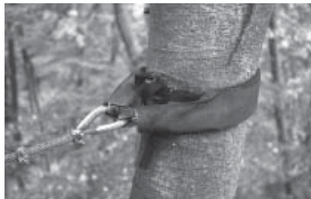
Figure 8.15 Left: Drawing of Osnabrück Double Belt System with an inner belt fixed to the stem (1) and a strong retaining outer belt (2). Right: Photo of the Osnabrück Double Belt System (Stobbe, Dujesiefken, & Schröder, 2000)
