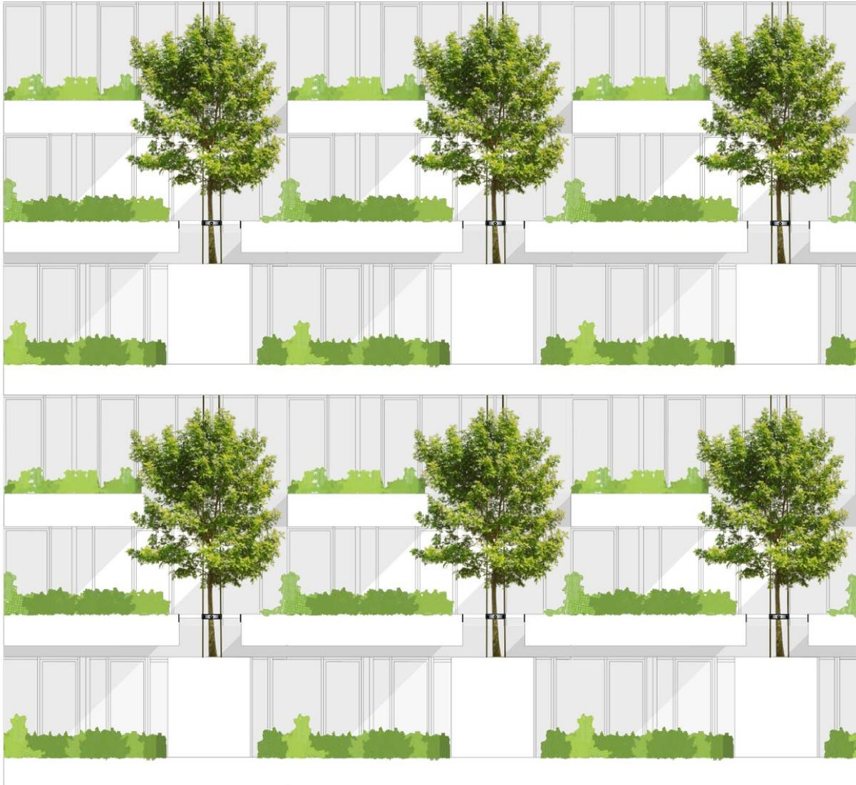
*Figure 8.5 Front view of Wonderwoods facade with plant containers connected to single trees*
