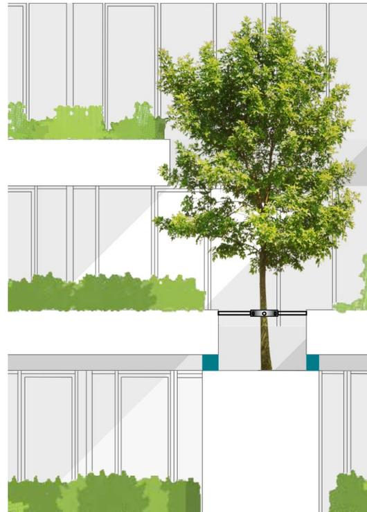
Figure 8.28 Front view of the *Wonderwoods* design, the blue blocks indicate the temporary support system
