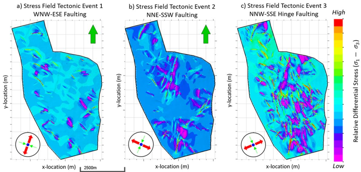
**Figure 4:** a-c) The modelled local differential stress field for each subsequent tectonic event respectively. The applied stress regimes are inversely calculated using the fracture and fault data.
