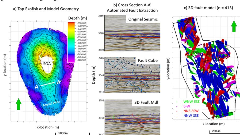
**Figure 1:** a) Model geometry and top Ekofisk horizon, which highlights the dome structure of the Ekofisk field. b) Cross section A-A', depicting the original seismic, the extracted fault cube and the faults included in the fault model. c) The 3D fault model.
