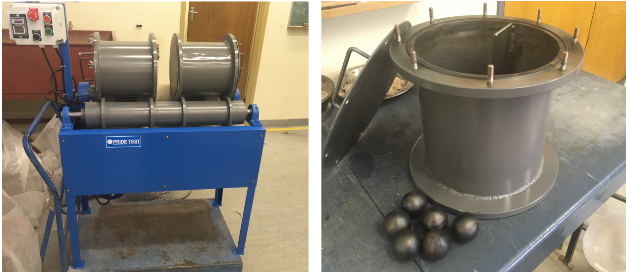
Figure 2.16: Double barrel durability mill at Stellenbosch University
