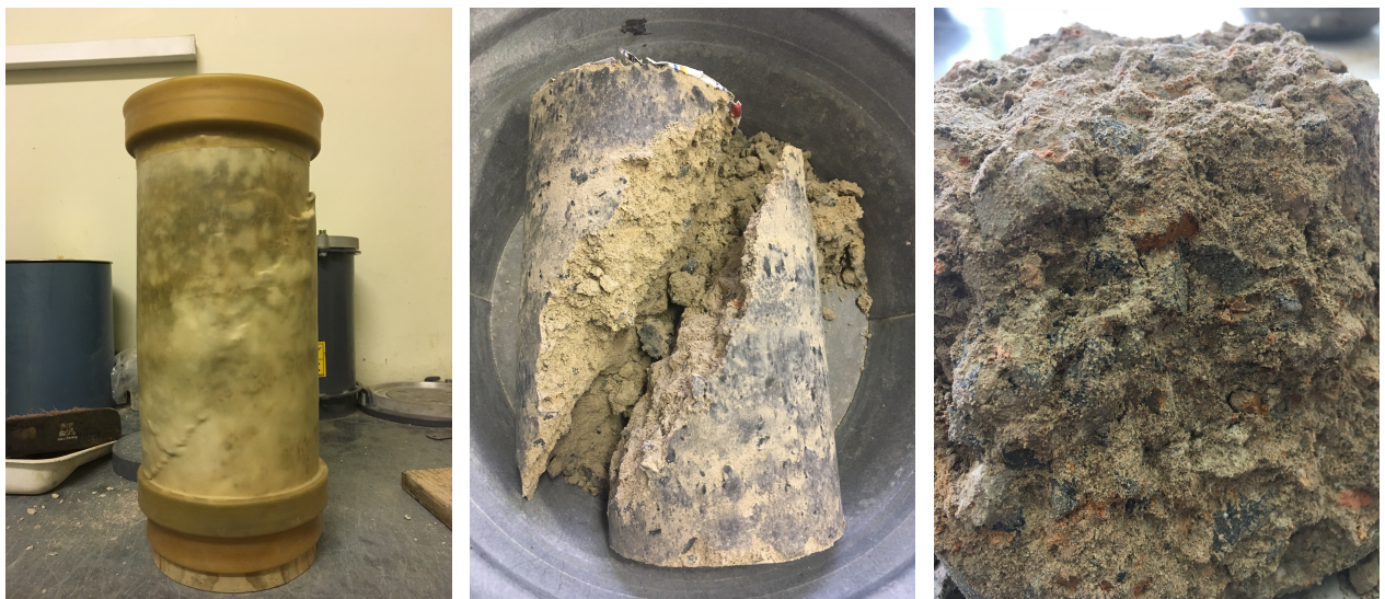
Figure 4.5: Typical shear failure observed in recycled aggregates
