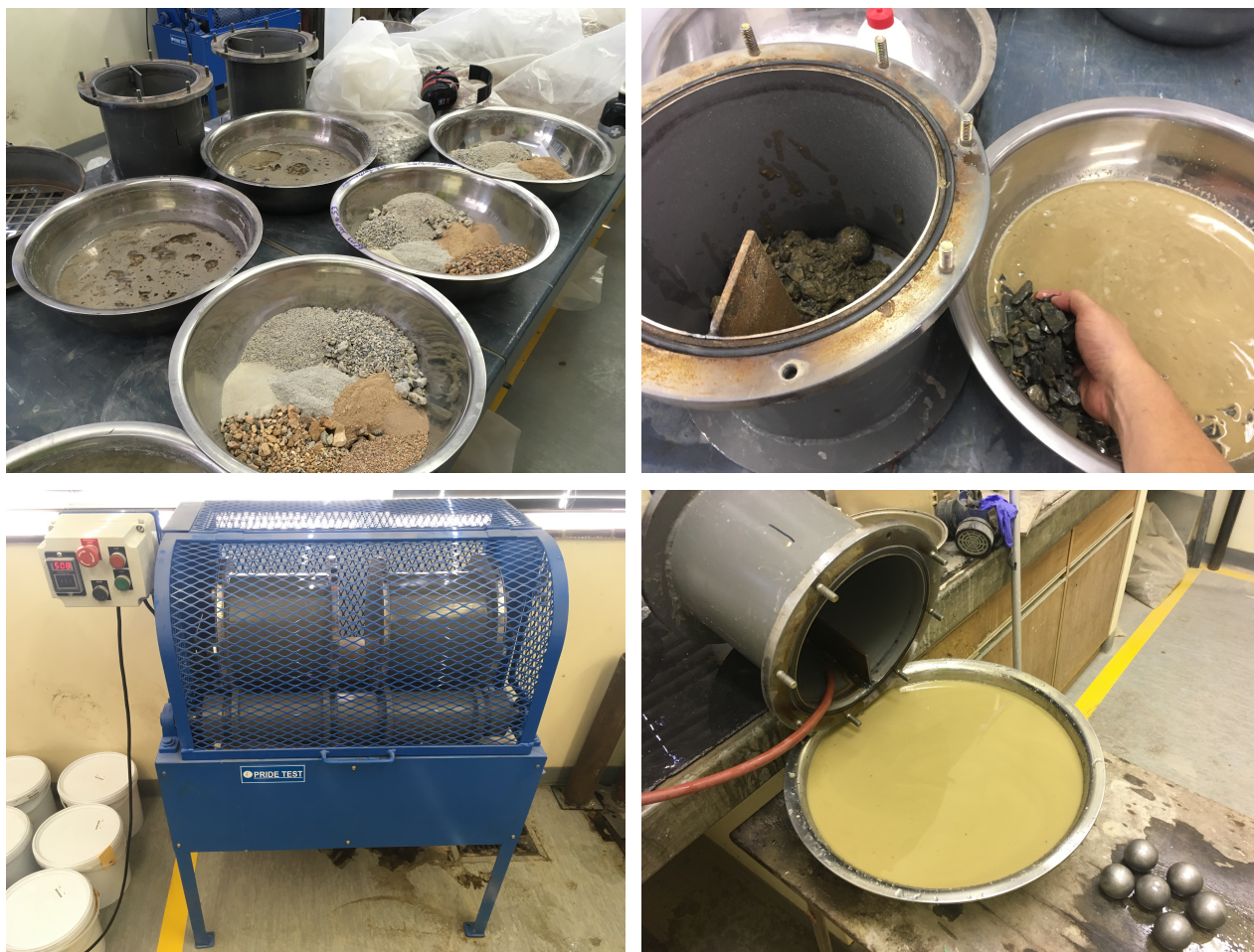
Figure 3.9: Durability milling: Soaking of the materials and loading, milling and washing out the drums
