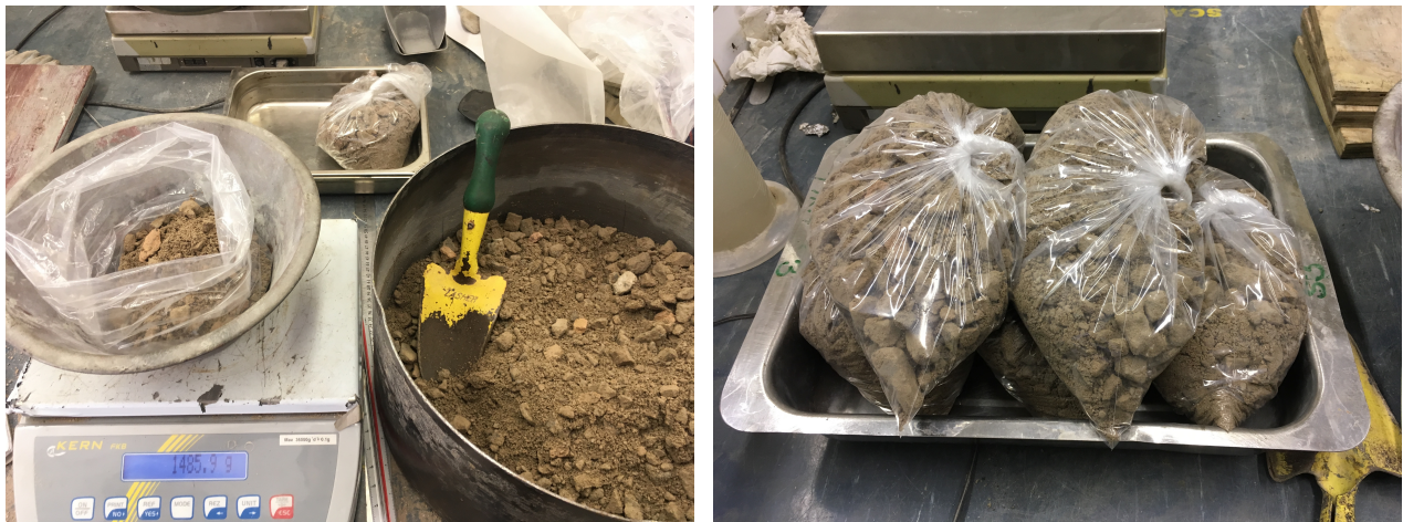
Figure 3.11: Weighing aggregates after mixing in five equal portions
