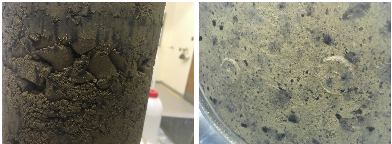
Figure 3.14: Specimen detailing Left: Without scraping the edges with the spatula Right: Uneven compaction plate
