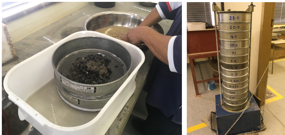
Figure 3.19: Left: Washing of the aggregates Right: Vibrating sieve tower
