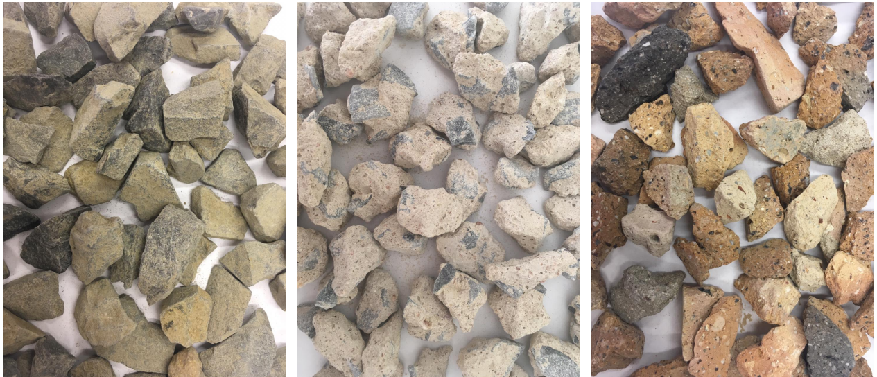
Figure 3.3: Material fractions 14 mm Left: G2 Middle: RCA Right: RCM
