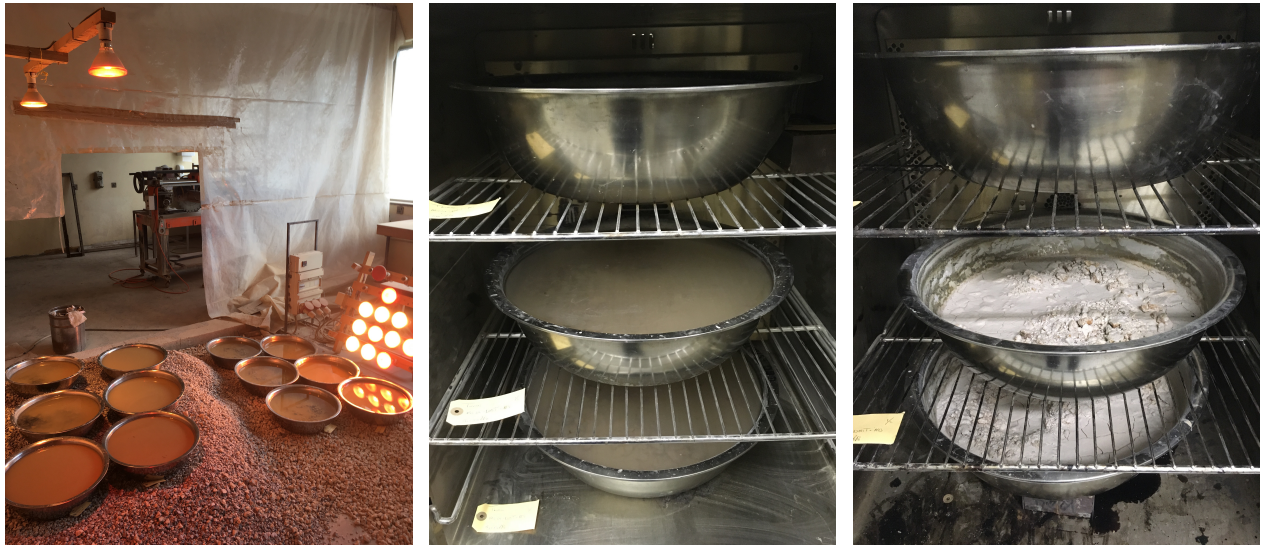
Figure 3.10: Drying process Left: Pre drying if oven capacity is exceeded Middle: Milled materials before drying Right: Milled materials after drying
