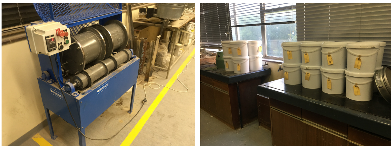
Figure 3.8: Left: Double barrel durability mill at Stellenbosch University Right: Buckets in line for sieving
