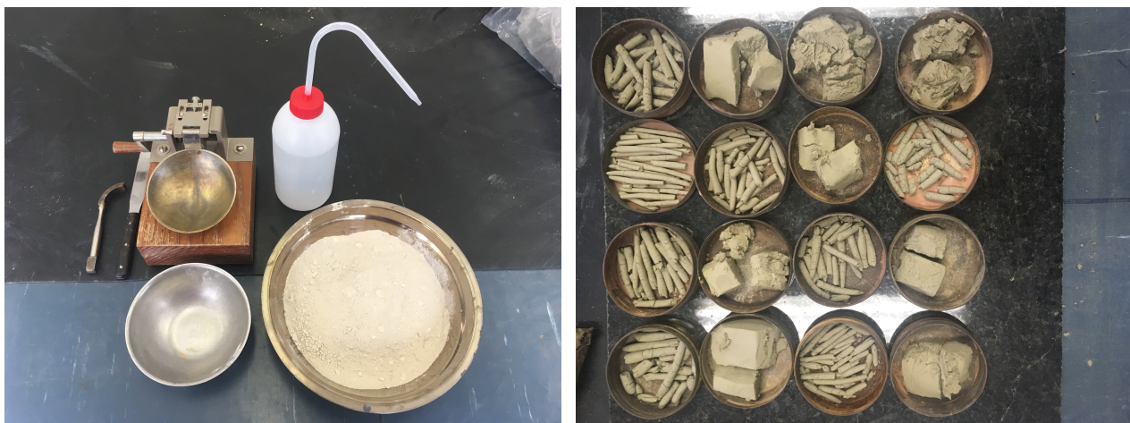
Figure 3.20: Left: PI test equipment Right: Tested samples for Liquid and Plastic Limits
