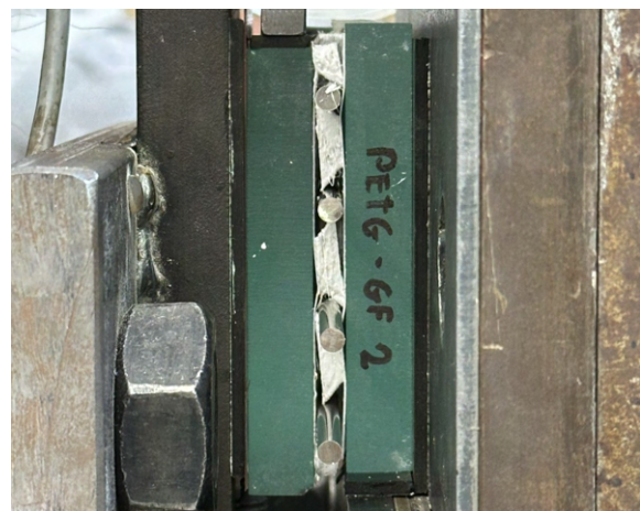
(b) Advanced wedging behaviour near peak load, showing increased key engagement and local deformation
