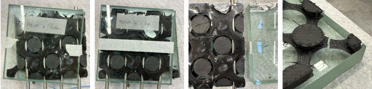
Figure E.28: Specimen S8 — PET-CF, Geometry 4 after testing
