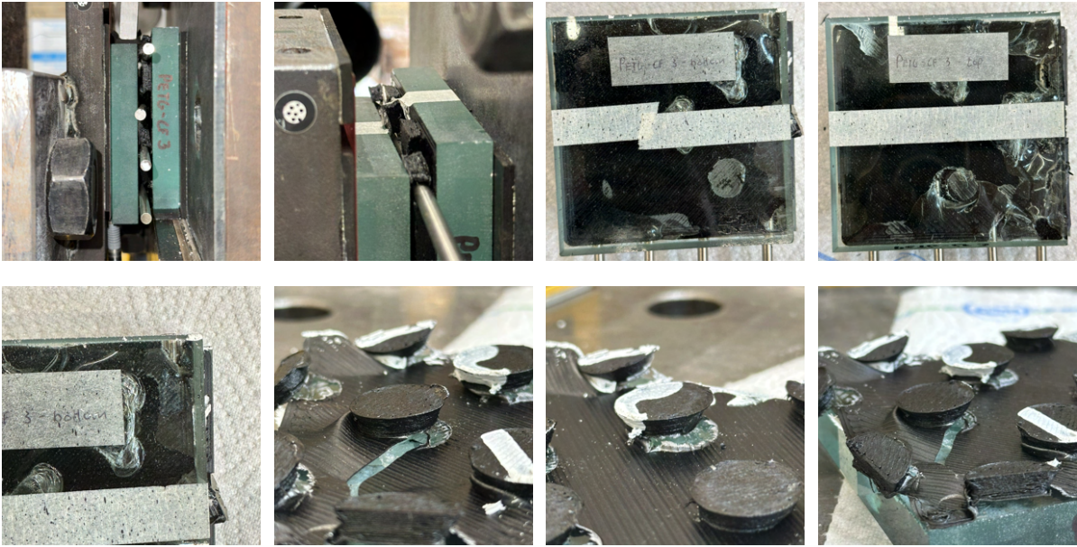
Figure E.13: Specimen S3 — PETG-CF, Geometry 3 after testing
