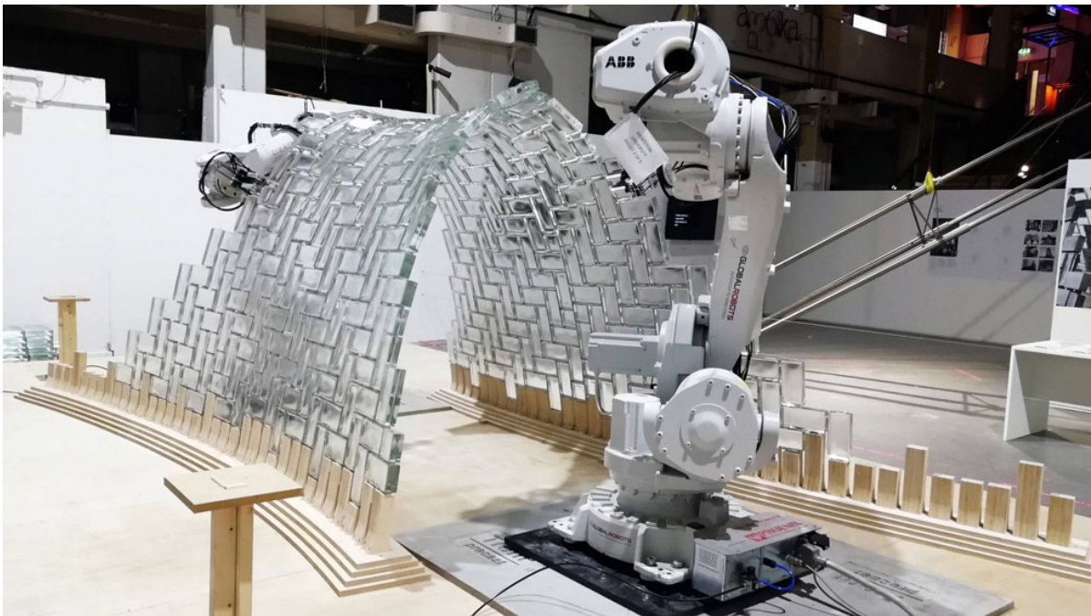
Figure 3.3: The Glass Vault , a robotically assembled cast-glass brick vault used as a reference case for this research. Image credit: Maciej Grzeskowiak
