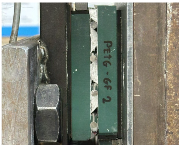
(a) Initial engagement of the interlocking keys during shear loading, showing limited wedging and deformation prior to peak load
