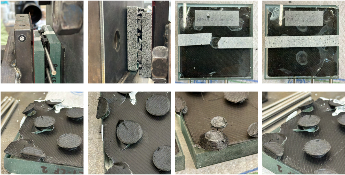
Figure E.22: Specimen S6 — PET-CF, Geometry 2 after testing
