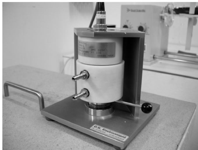
Figure 3.1 – Rotronic station for RH measurement
