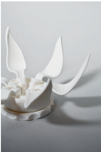
Used too much force which broke upper from base
