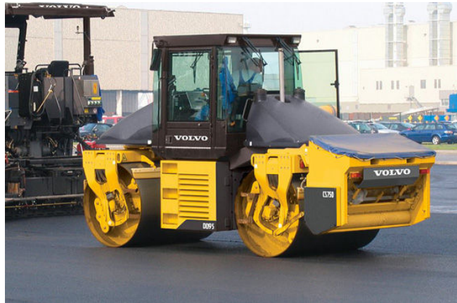
Figure 1-1: Roll Over Protection for Compactor: The roll over protection structure can be seen over the drivers seat
