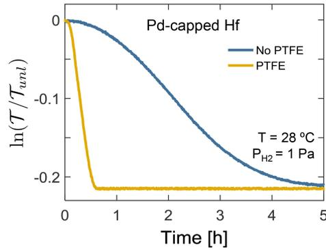
**Fig. 4.** (Color online) Effect of sputtered PTFE on the kinetic properties of two 40 nm Hf thin films capped with a 10 nm Pd layer with and without an additional PTFE layer. The two films were simultaneously exposed to a constant hydrogen pressure of  $P_{\text{H}_2} = 1$  Pa at  $T = 28$  °C. The white-light optical transmission  $\mathcal{T}$  is normalized to the transmission of the unloaded states  $\mathcal{T}_{\text{unl}}$ . Data adapted from Boelsma et al. (2017).<sup>29)</sup>
