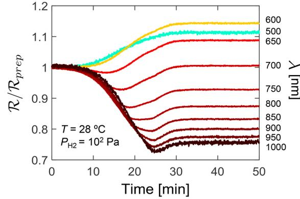
**Fig. 9.** (Color online) Wavelength dependence of the changes in reflectivity of a Pd-capped 40 nm Ta thin film with a 4 nm Ti adhesion layer. The thin film was exposed to a constant hydrogen pressure of  $P_{\text{H}_2} = 100$  Pa at room temperature. The reflectance  $\mathcal{R}$  is measured relative to the reflectance of the as-prepared state  $\mathcal{R}_{\text{prep}}$ . Data adapted from Boelsma (2017).<sup>55)</sup>
