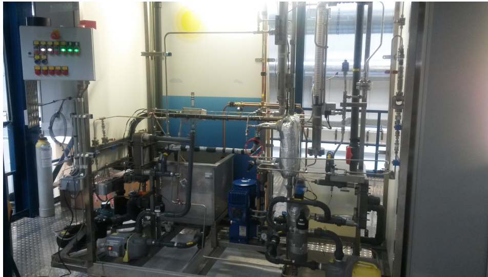
Figure 5.1: The OTEC Demo. The big steel tank on the left is the warm water tank and the plastic one on the right is the cold water tank. The recuperator is wrapped in silver insulation and insulated pipes go from the recuperator to the evaporator on the left and to the condenser on the right. The separator is a narrow vertical tank situated above the recuperator in the figure. The working fluid pump is the blue pump in the middle of the figure and the water pumps are the grey and yellow pumps in each corner.
