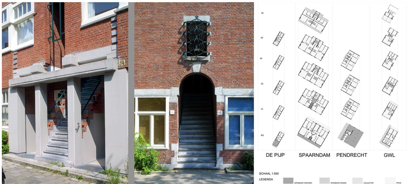
Figure 7. Grounded-ness, the tradition of the own front door. From left to right: Photographic examples of the own front door in in Amsterdam Zuid; comparison of Amsterdam access types ranging from De Pijp, Spaarndammerbuurt, Pendrecht, and GWL terrain in Amsterdam and Rotterdam. Source: Authors.
