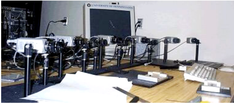
Figure 2.16: An array of cameras for multiview capture [42]
