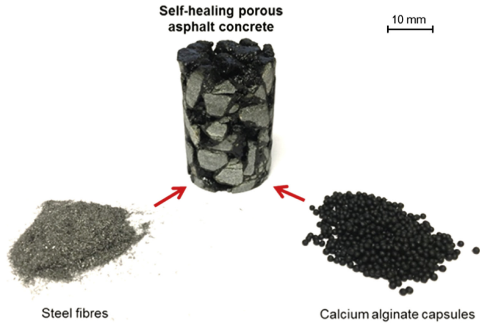
Fig. 3. Steel fibres and calcium alginate capsules used in self-healing porous asphalt concrete.
