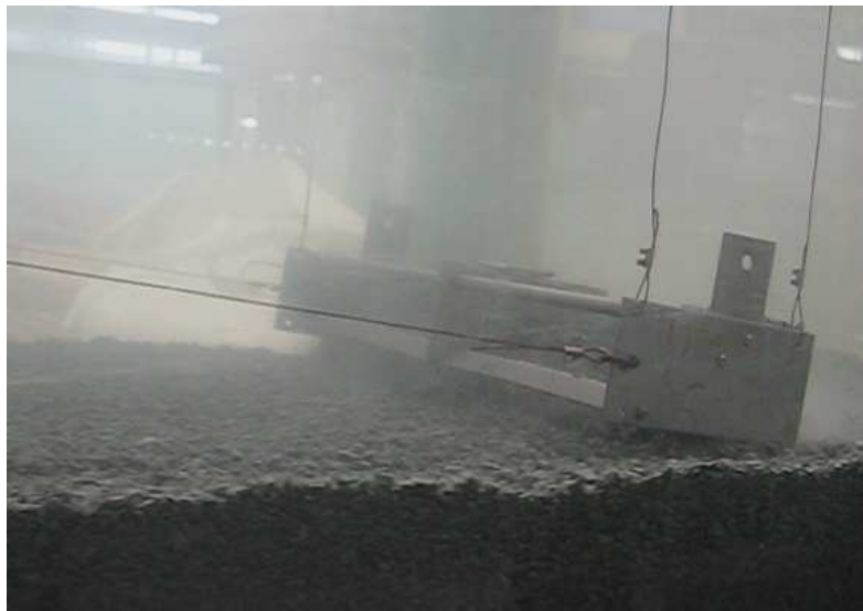
Figure 6.1 Plough suspension during a transporting experiment in cobbles ( D_{50} = 5,2 \text{ mm} )
