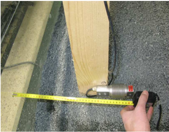
Figure 5.5 Force measurement tools: Load cell, Volt meter
