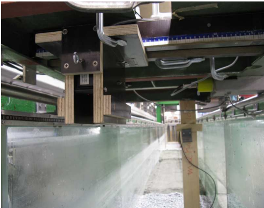
Figure 5.6 Geometry measurement tools: Single beam laser, distance "pulse ticker"
