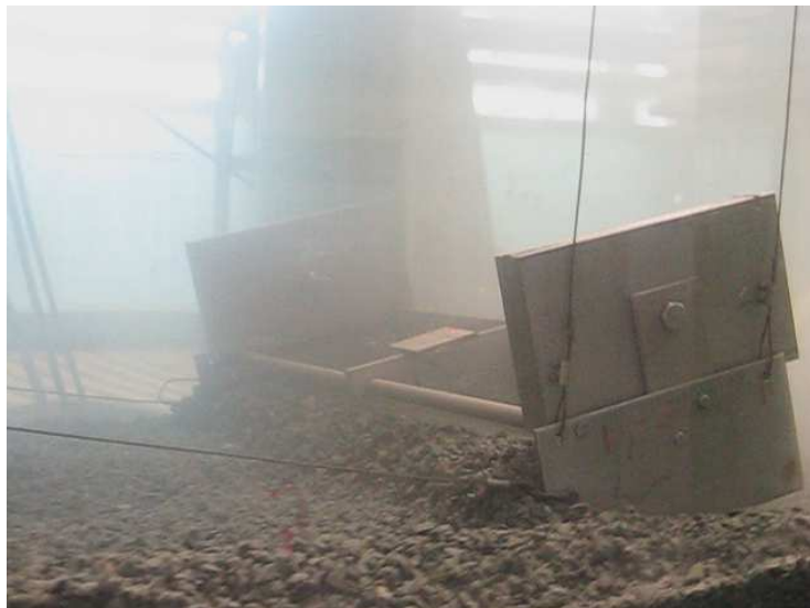
Figure 6.11 Maximum penetration during a cutting experiment in cobbles ( D_{50} = 5,2 \text{ mm} )
