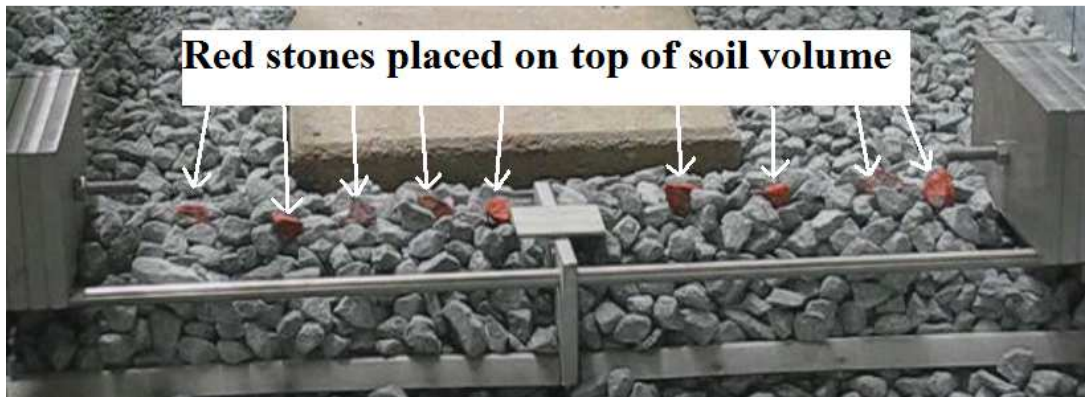
Figure 6.2 Testing stone movement by placing red stones on top of the soil volume
