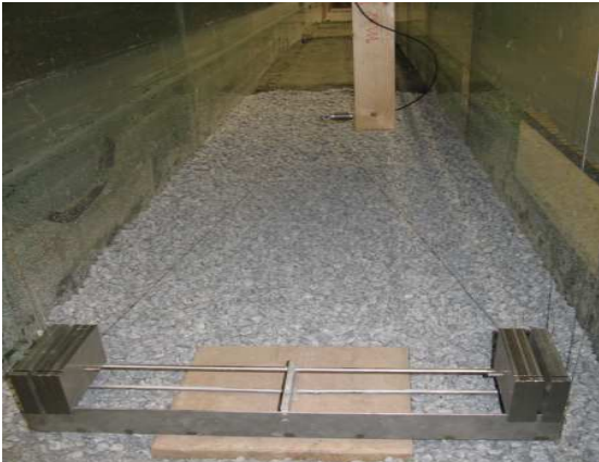
Figure 5.7 Suspension measurement tools: height calibrated bricks , turn buckels
