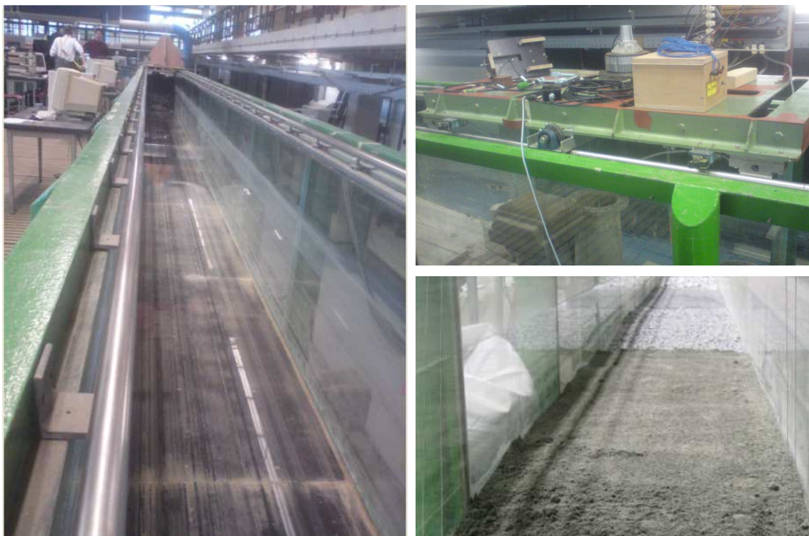
Figure 5.1 Speurwerkgoot: flume (left), drag mechanism (right top)
