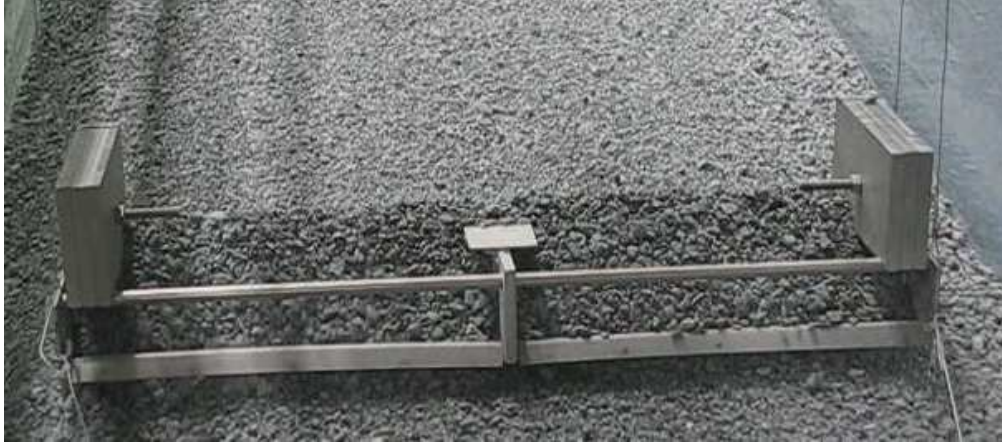
Figure 6.24 Triangular soil volume in front of rear blade for a stationary cutting situation with h_i = 0
