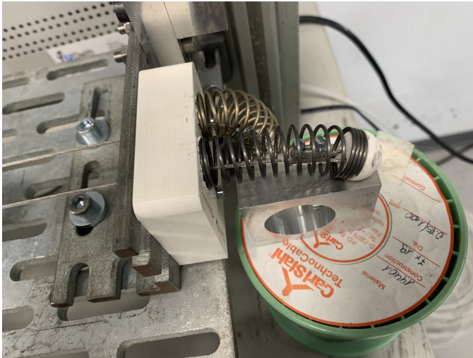
Fig. 29. Finger bending test picture. In the picture there can be seen that one finger is bend and the other finger is extended, when taking a closer look it is visible that the windings of the extended finger are closer together because of the pulling force exerted on the cable.
