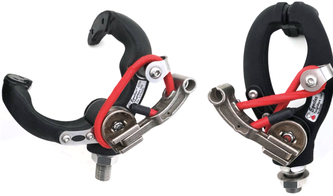
Fig. 16. The Equilux by ToughWare, the figure shows the clamp respectively in its voluntary closing and voluntary opening position. By flipping the large metal lever from one side to the other the modes can be switched, the actual switching happens because of the repositioning of the elastic band pulling force from one side of the joint to the other side of the joint. [19]
