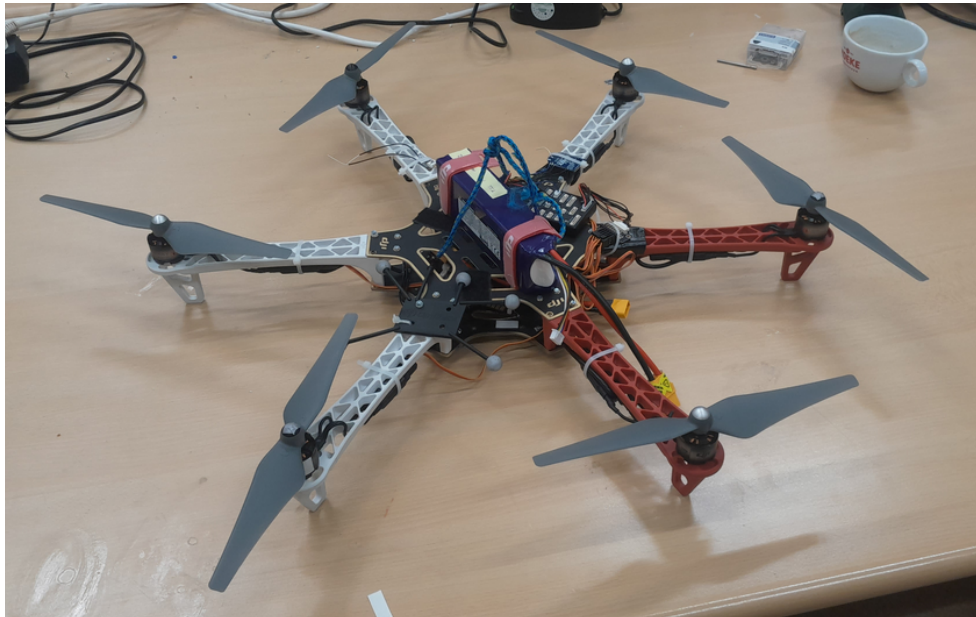
Figure 5.2: Flame Wheel Hexacopter, read-to-fly. Note the infrared markers on one of the arms and on some propellers. The centered attachment for a vertical safety rope is also visible.
