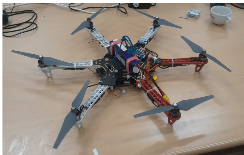
Figure 3. Hexacopter test platform with battery, Pixhawk flight controller and reflective infra-red markers.
